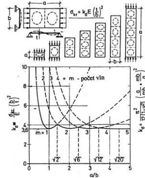
Fig.12 Number of waves on the skin within the compressive loading
