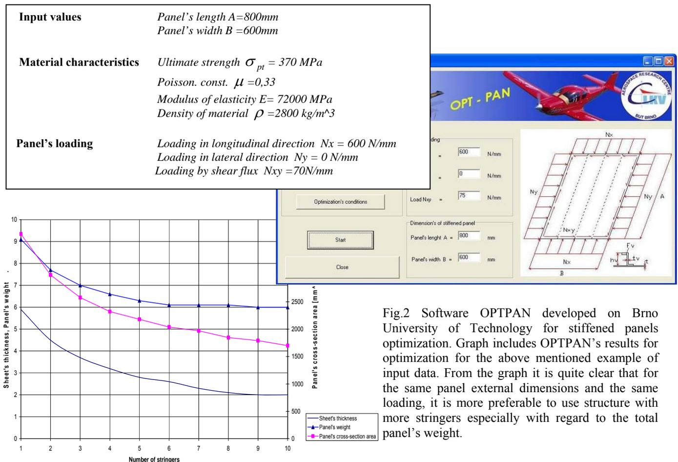
Fig.2 Software OPTPAN developed on Brno University of Technology for stiffened panels optimization. Graph includes OPTPAN's results for optimization for the above mentioned example of input data. From the graph it is quite clear that for the same panel external dimensions and the same loading, it is more preferable to use structure with more stringers especially with regard to the total panel's weight.
