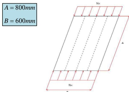
Fig.7 External panel's dimensions and loading type
