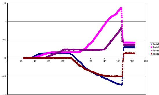
Fig.16 Relation between aripots deviation and panel's loading. The point of buckling start is clear.
