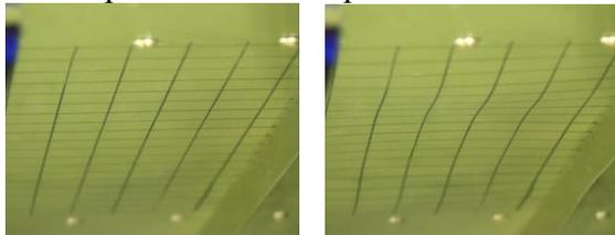
Fig.11 Unbuckled vs. buckled stiffened panel
