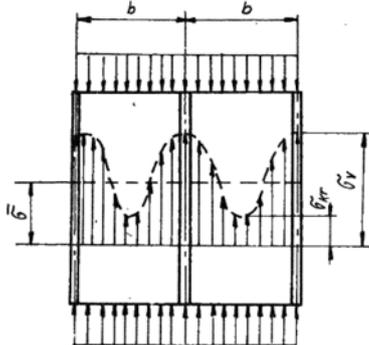
Fig.23 The real stress distribution along the cross section area of the stiffened panel
