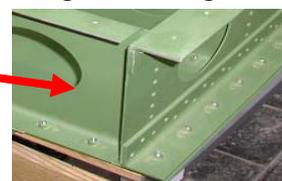
buckling and post buckling behaviour of the stiffened panel. Riveting nuts for easier panel's exchange are attached in the flanges of the ribs and flanges of the spar. It is also possible to fasten two stiffened panels on one box (both sides are ready for panel's clamping) at one moment by threads. It
