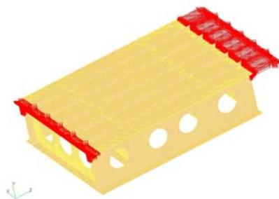
Fig.5 Boundary condition of stiffened panel and testing box
