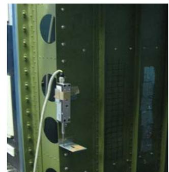
Fig.19 Determination of loading distribution by drift meters
