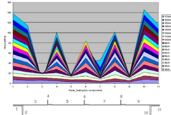
Fig.22 The real stress distribution along the cross section area of the stiffened panel and testing box
