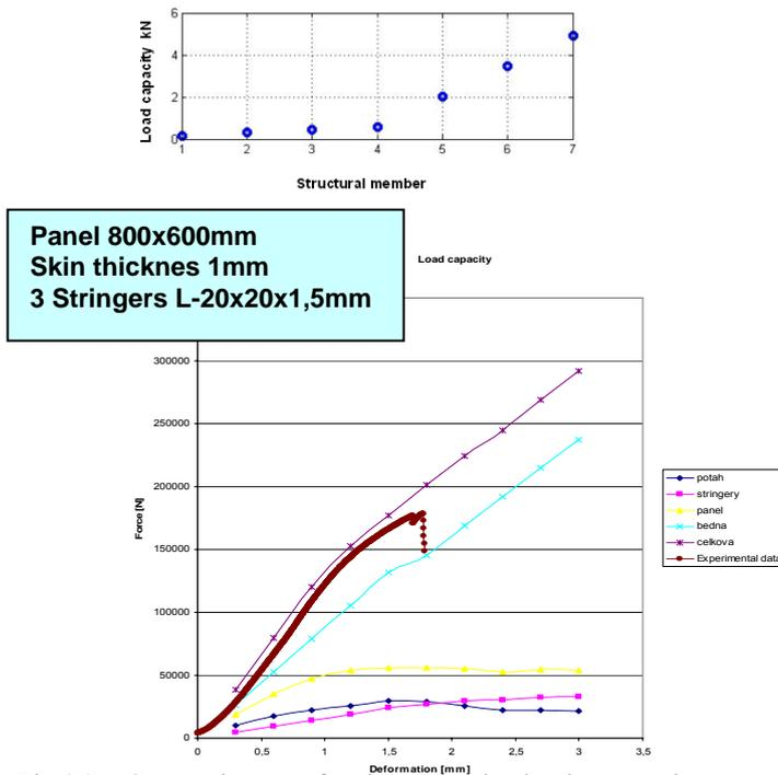
Fig.24 Comparison of the panel load capacity (approximately 50kN) and the total load capacity (180kN) for input data was made. The results from all three methods seem to be very similar.
