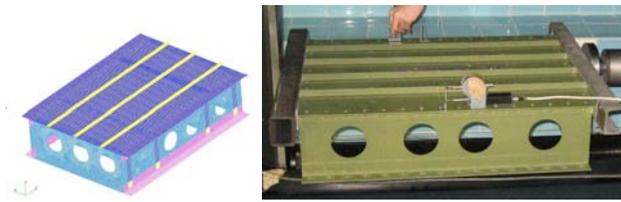
Fig.4 Testing box including stiffened panel (Modeled vs. Real)
