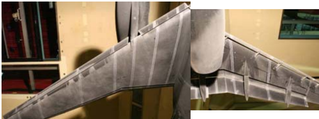
Fig. 4 China-clay visualization of boundary layer transition at \alpha = 10^\circ (Black: Laminar, White: Turbulent)
