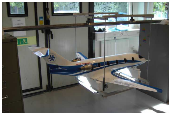
Fig.6. Raven inertia measuring.
