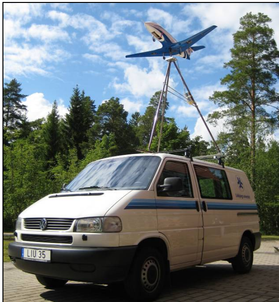
Fig. 7. Raven mounted on car top test rig.
