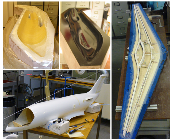
Fig. 4. Different stages in manufacturing.
