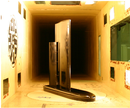
Figure 2. Simplified HLD model in 2.0 x 2.0m wind tunnel (JAXA-LWT2).
