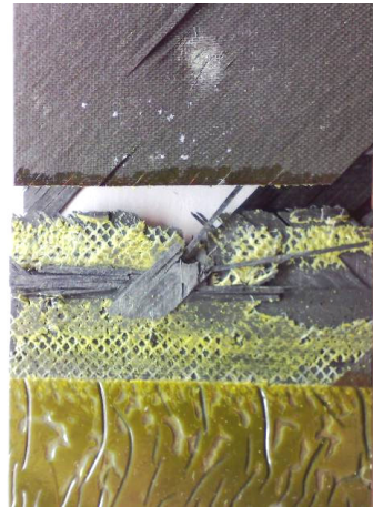
Figure 3: Failed specimen showing debonding and a small amount of composite failure in the 45° and 90° plies
