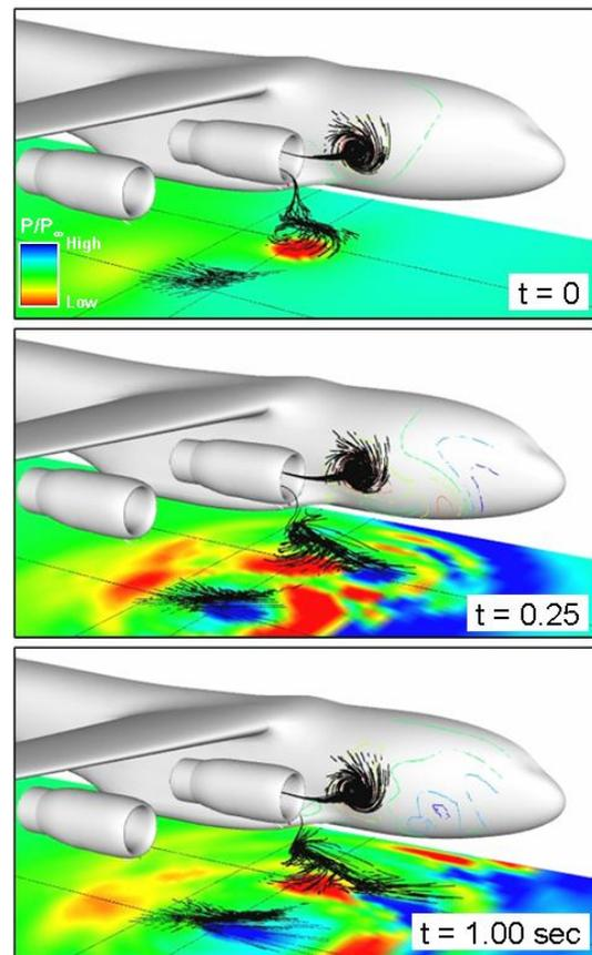
**Fig. 2: Flow development due to pulsed jet actuation (pressure contours on the ground plane and particle traces)**
