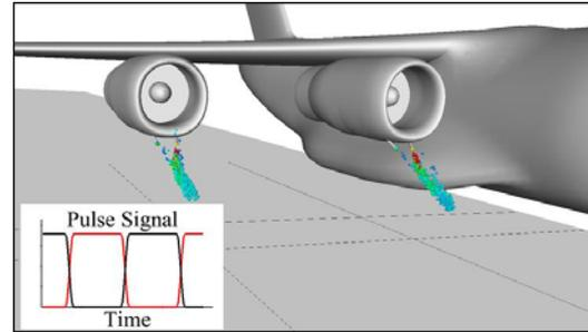
**Fig. 1: Pulsed jet ejection described by particles released from actuator nozzles**
