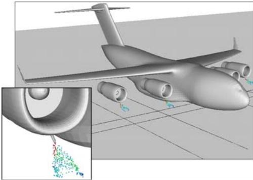
**Fig. 3: Sprinkler jet ejection described by particles released during the first five cycles (0.036 sec) from start of actuation**
