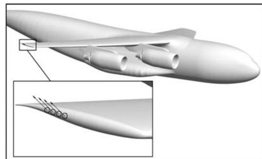
Fig. 5: System for the control of wing vortex
