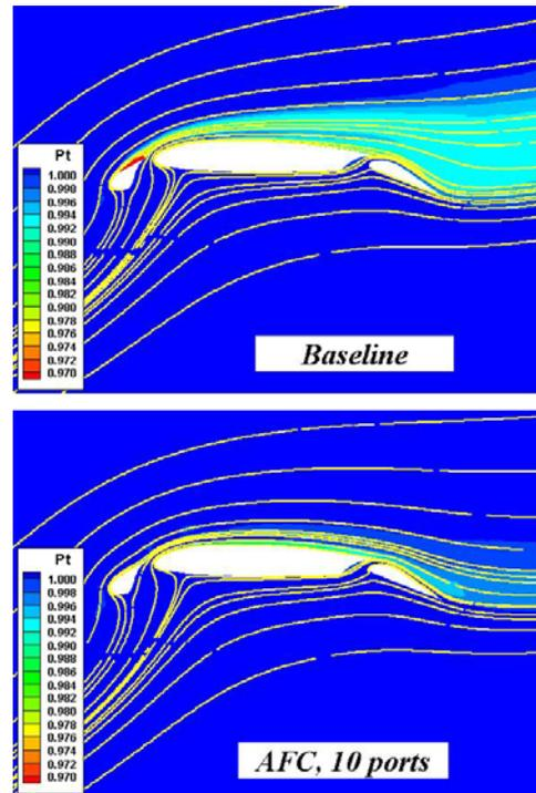
Fig. 12: Impact of AFC on flow structure of the conventional high-lift system (time-averaged total-pressure,  $\alpha=19^\circ$ )
