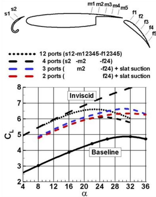
Fig. 13: AFC for advanced wing section (landing configuration,  $\delta_{flap} = 50^\circ$ )
