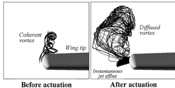
**Fig. 6: Near-field wing tip flow structure before and after actuation (front view)**
