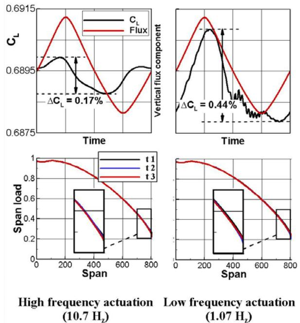
Fig. 8: Lift response and instantaneous wing load distributions due to actuation
