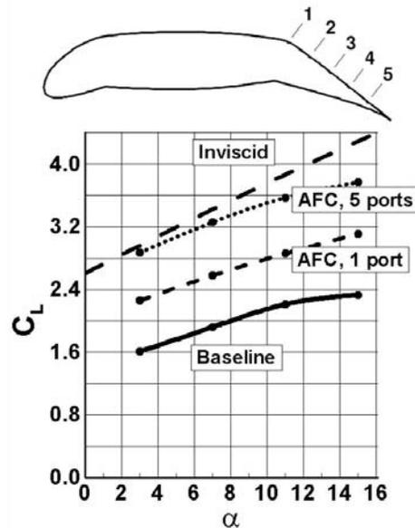
Fig. 9: Lift augmentation due to distributed flow control – simple hinge flap
