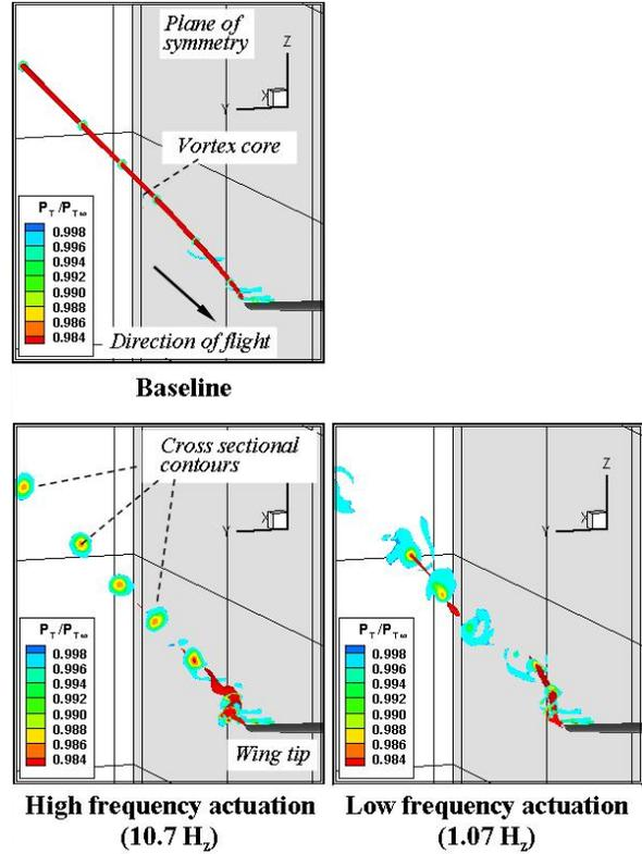
Fig. 7: Trailing vortex before and after application of flow control (total pressure)
