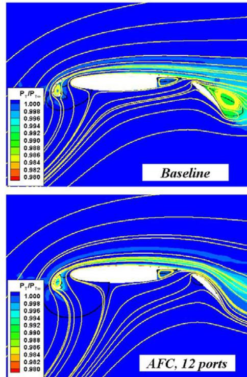
Fig. 14: Time-averaged total-pressure field showing impact of AFC on confluent viscous layers of the advanced wing section (time-averaged total-pressure,  $\alpha = 22^\circ$ )
