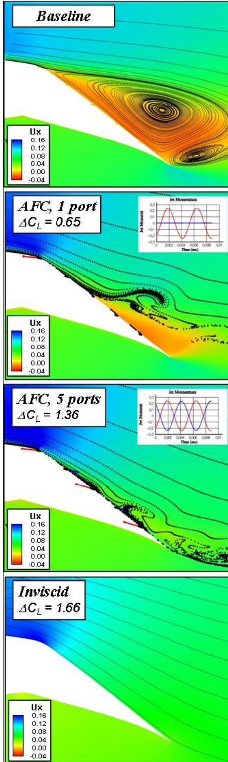
Fig. 10: Instantaneous flow field description for a simple hinge flap system (streamwise component of velocity,  $\alpha=11^\circ$ )
