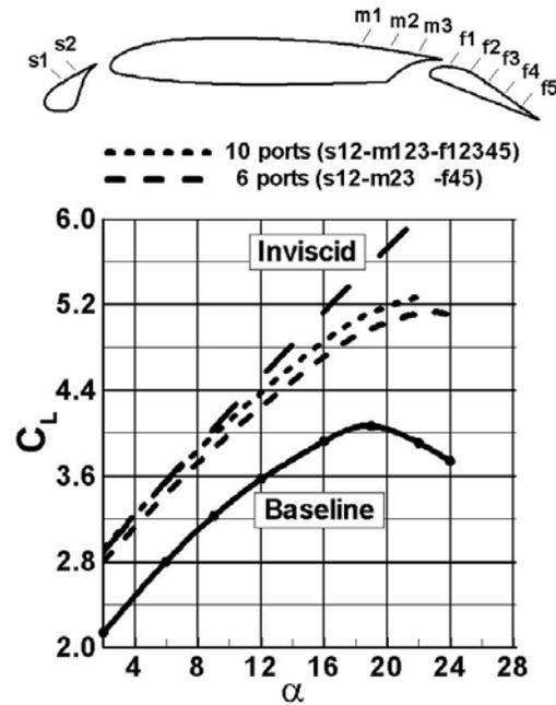
Fig. 11: Effect of AFC application at each element of the conventional high-lift wing section (representative takeoff configuration,  $\delta_{flap} = 24^\circ$ )
