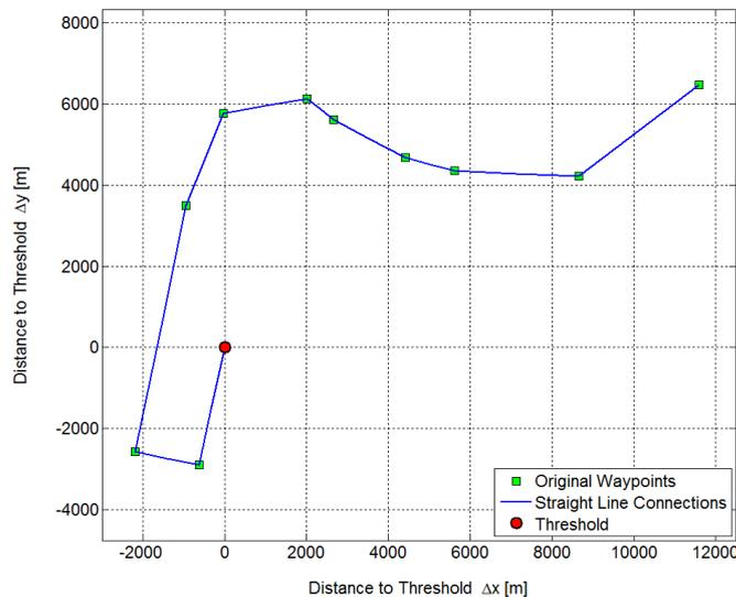
Fig. 5 Basic flight path with original waypoints connected by straight lines
