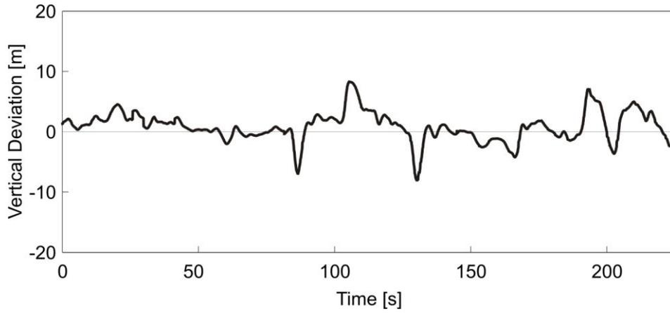
Fig. 15 Vertical deviation from command flight path
