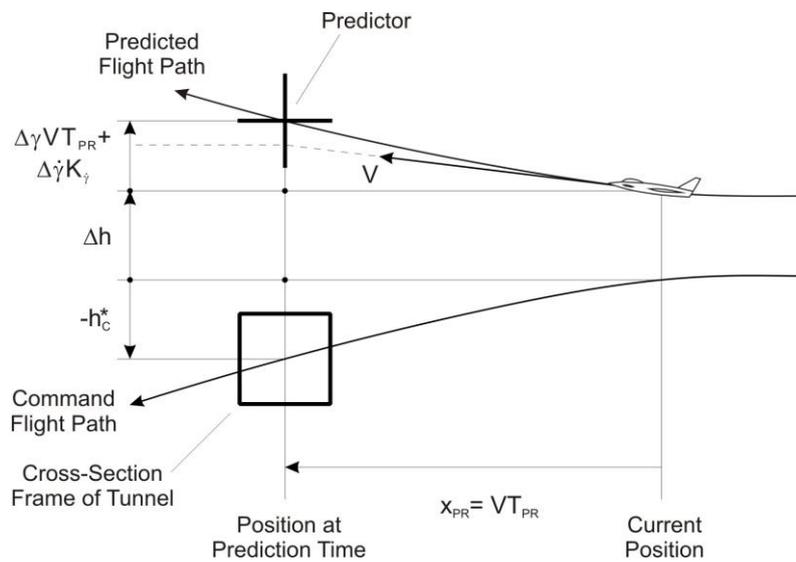
Fig. 11 Predictor and longitudinal flight path continuation
