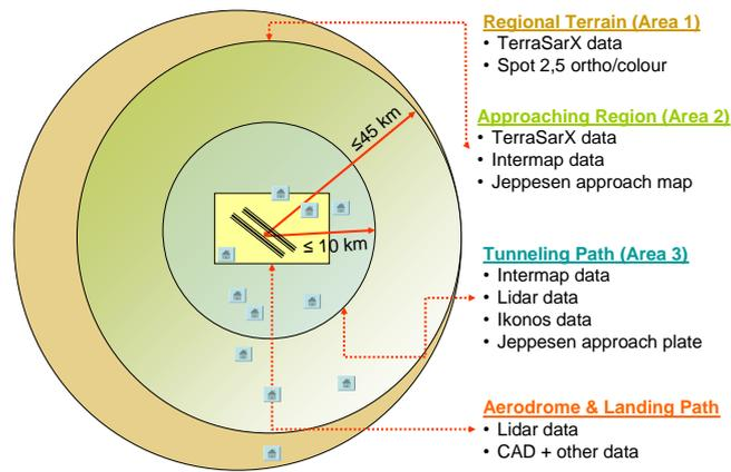
Fig. 3 GIS data sources used for areas with different distances to airport
