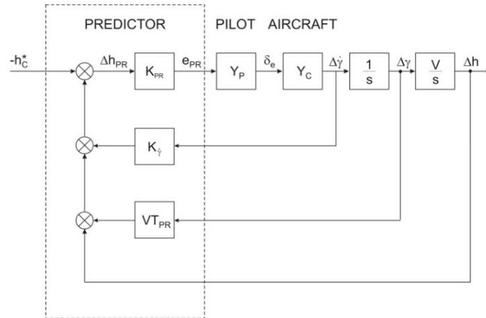
Fig. 12 Block diagram for longitudinal predictor
