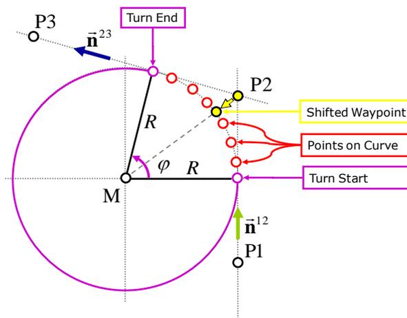
Fig. 7 Curved trajectory segment with shifted waypoint
