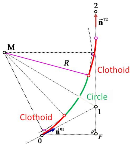
Fig. 8 Clothoid segments at beginning and end of a curve
