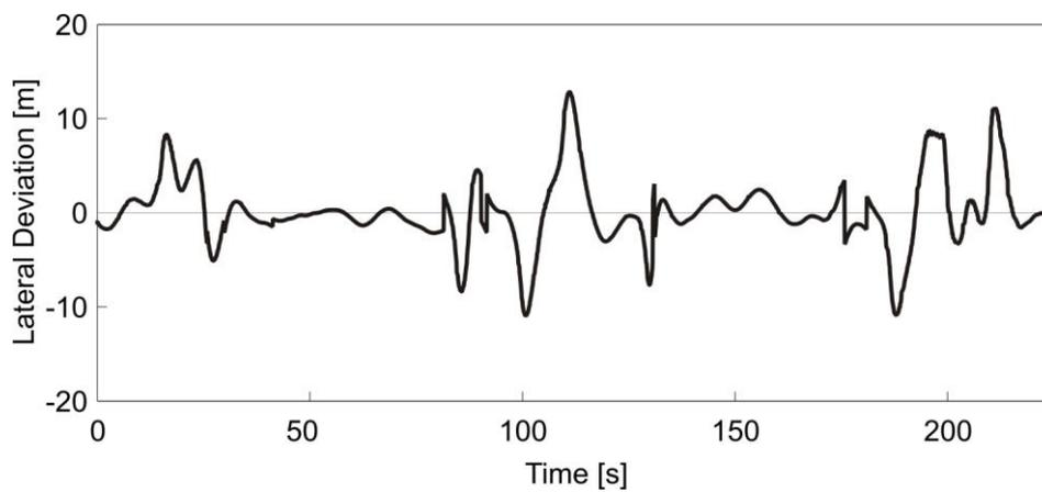
Fig. 14 Lateral deviation from command flight path
