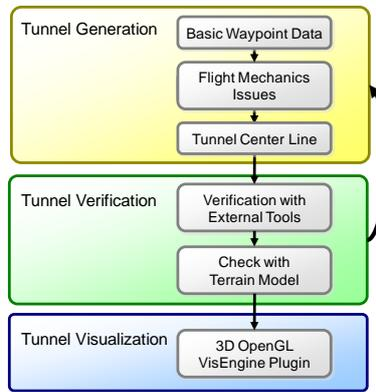
Fig. 4 Tunnel generation process
