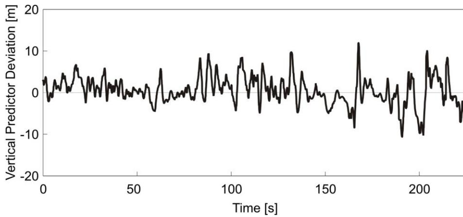
Fig. 17 Vertical predictor deviation from command flight path
