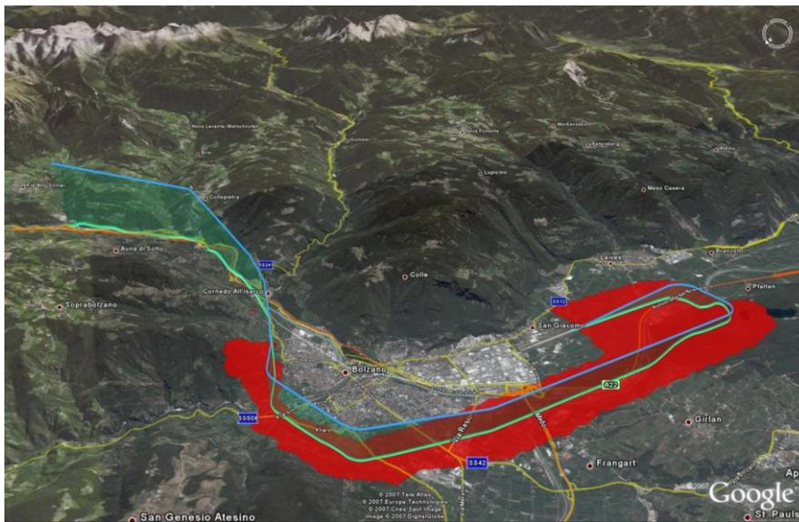
Fig. 10 Tunnel and ground track of approach trajectory to Bolzano airport
