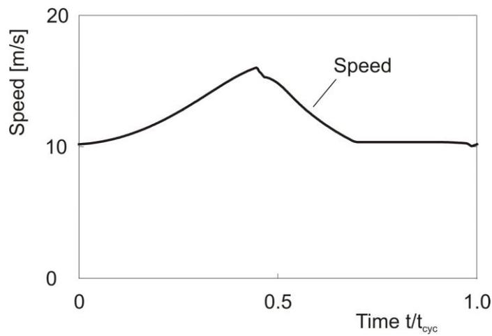
Fig. 7 Optimal speed time history for minimizing required battery capacity
