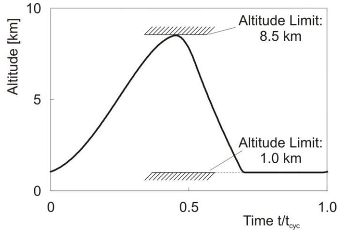
Fig. 6 Optimal altitude time history for battery energy storage minimization
