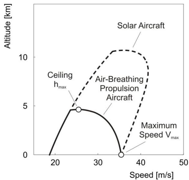
Fig. 4 Flight envelope of an aircraft with an air-breathing propulsion system
