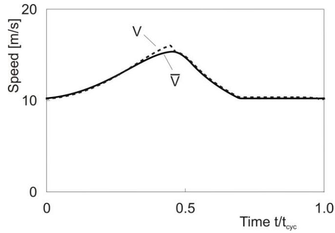
Fig. 9 Optimal speed from trajectory optimization ( $V$ ) and speed for minimum power required in steady-state flight ( $\bar{V}$ )
