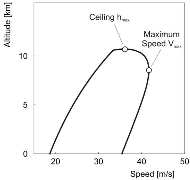
Fig. 3 Flight envelope of a solar aircraft
