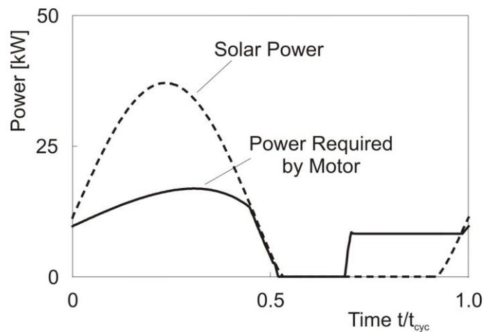
Fig. 8 Solar and engine power for battery energy storage minimization
