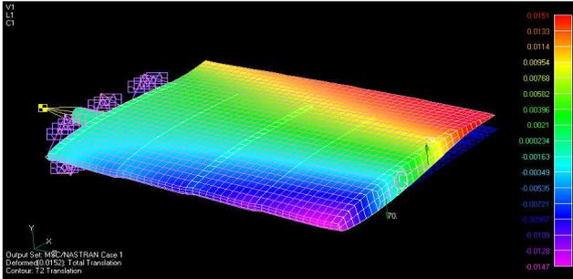
Fig. 11. Aeroelastic fin displacements under actuators action.
