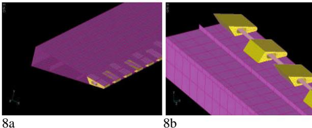
Fig. 8a-b Swivel concept applied on the TE of the MT4.
