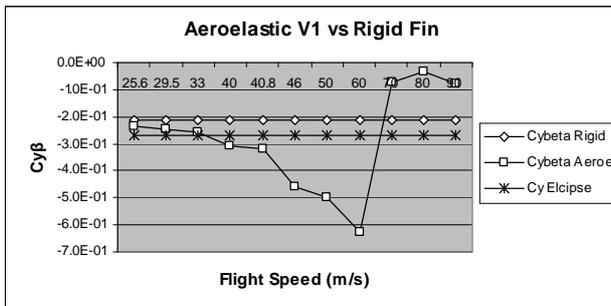
Fig. 12 Comparison of  $C_{y\beta}$  coefficients between GRAF and conventional designs.
