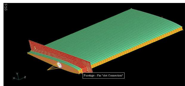
Fig. 5. Fin inserted into the “slot connection” (red).
