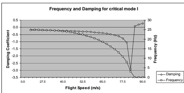
Fig. 16 Frequency and damping coefficients vs flight speeds.
