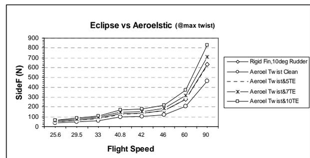
Fig. 10 Sideforce comparison between conventional and aeroelastic fin.
