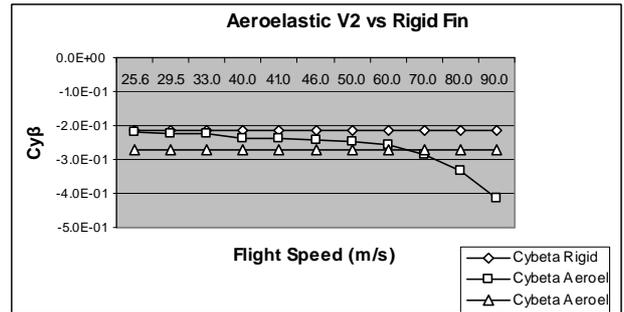
Fig. 13. Comparison of  $C_{y\beta}$  coefficients between GRAF and conventional designs.
