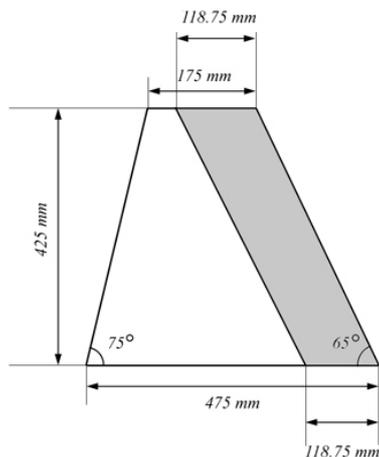
Fig. 4 Eclipse Fin Geometry
