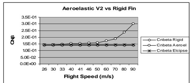
Fig. 15. Comparison of  $C_{N\beta}$  coefficients between GRAF and conventional designs.
