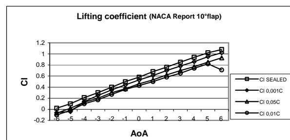
Fig.1 NACA 0009 Lifting Coefficient with sealed gap[13]
