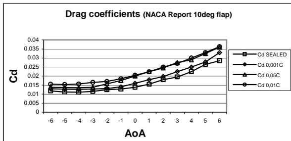
Fig.2 NACA 0009 Drag Coefficient with sealed gap [13]
