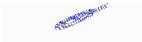
Fig. 9 Carbon Fiber Rib of the MT4 model
