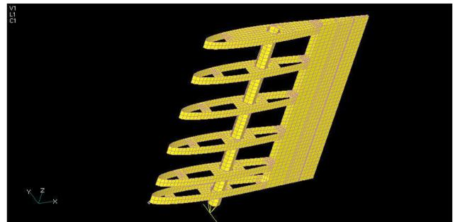
Fig. 7 GRAF-MT4: Ribs, flexible TE and carrying load beam.
