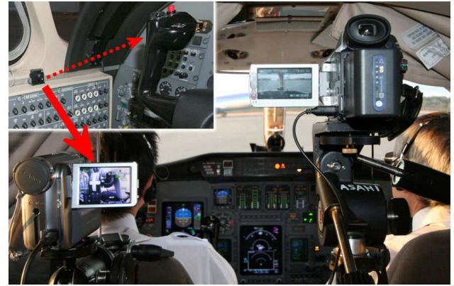
Fig. 4 The control command is recorded using a white cross marker on the column (left), the visual cues are recorded with the camera on the right.
