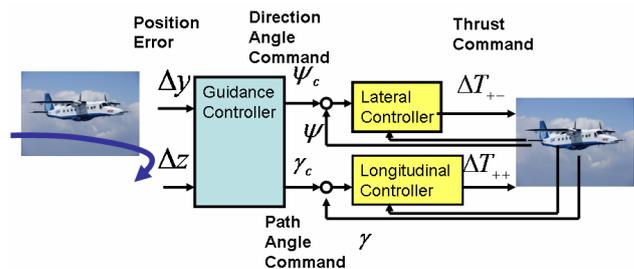
**Fig. 6** Engine power flight control system
