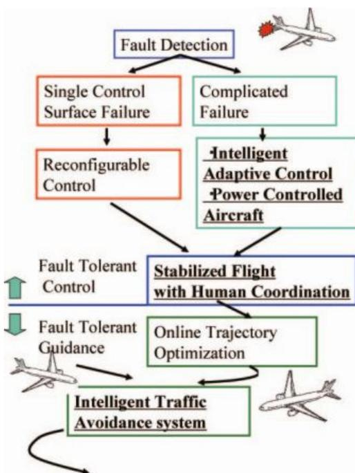
**Fig. 1** Block diagram of intelligent fault tolerant flight control system
