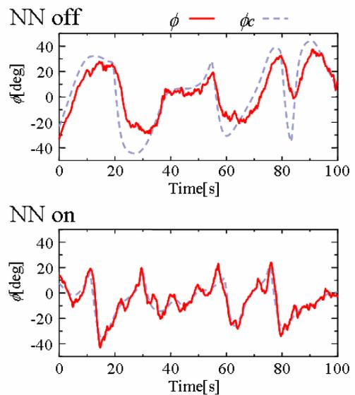
Fig. 13 Command bank angle and output data with and without NN
