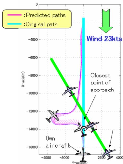
**Fig. 9** Optimal air collision avoidance system
