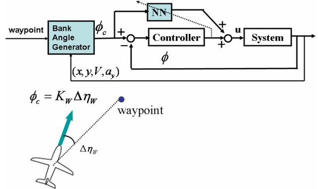
Fig. 11 Waypoint Tracking Controller with Neural Network
