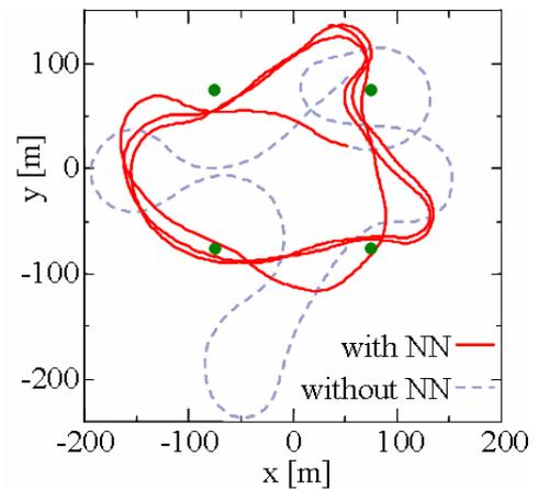
Fig. 12 Flight trajectories of UAV with and without NN
