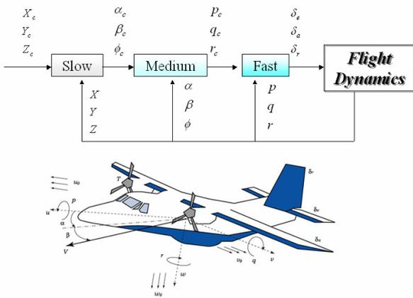
**Fig. 8** Nonlinear dynamic inversion with singular perturbation method
