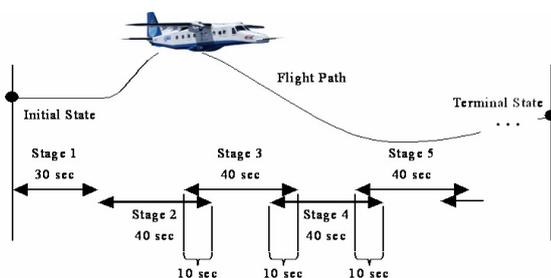
**Fig.7** Multistage division for online flight trajectory optimization
