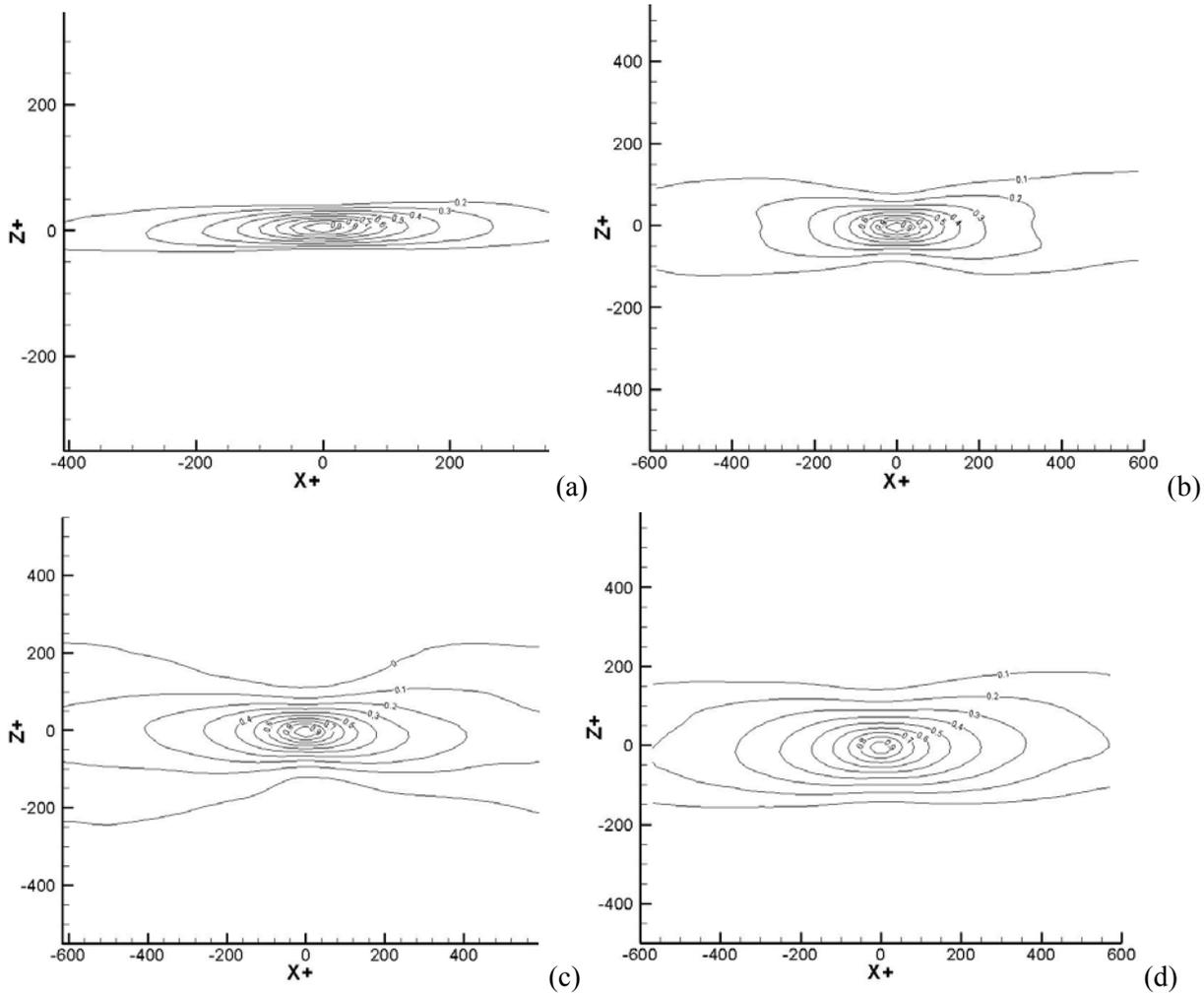
Fig.12 Two point streamwise velocity auto-correlation function in the plane  $y/\delta < 0.1$ . (a): smooth wall, (b): 2D wall, (c): 3D-0° wall, (d): 3D-45° wall.
