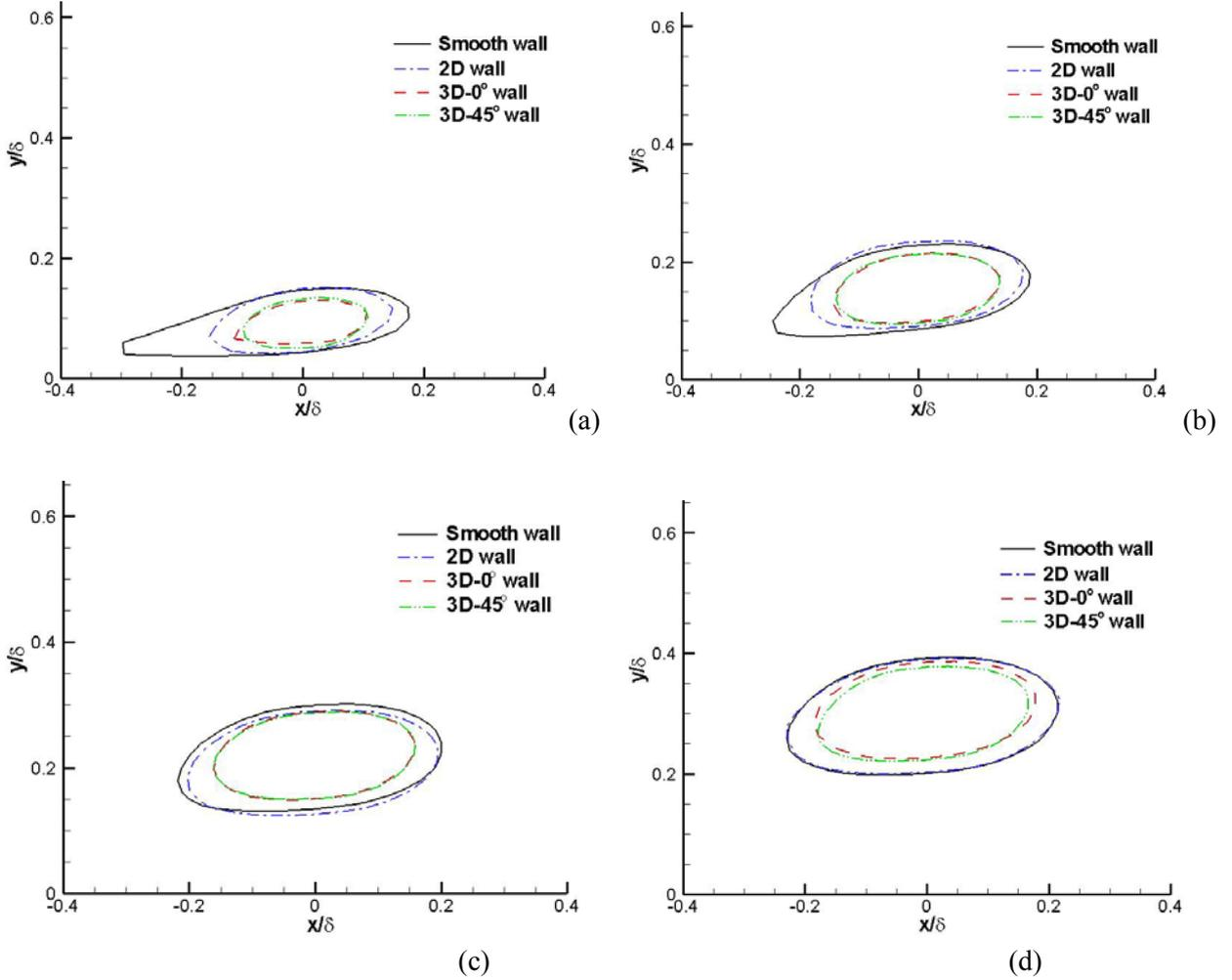
Fig. 9 Contours of constant values of the two point streamwise velocity auto-correlation function,  $\rho_{u'u'} = 0.6$ . (a):  $(y/\delta)_{\text{ref.}} = 0.1$ ; (b):  $(y/\delta)_{\text{ref.}} = 0.15$ ; (c):  $(y/\delta)_{\text{ref.}} = 0.2$ ; (d):  $(y/\delta)_{\text{ref.}} = 0.3$ .
