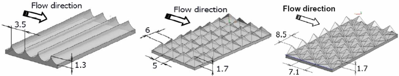
Fig.2 Roughness geometries. Dimensions in mm.
