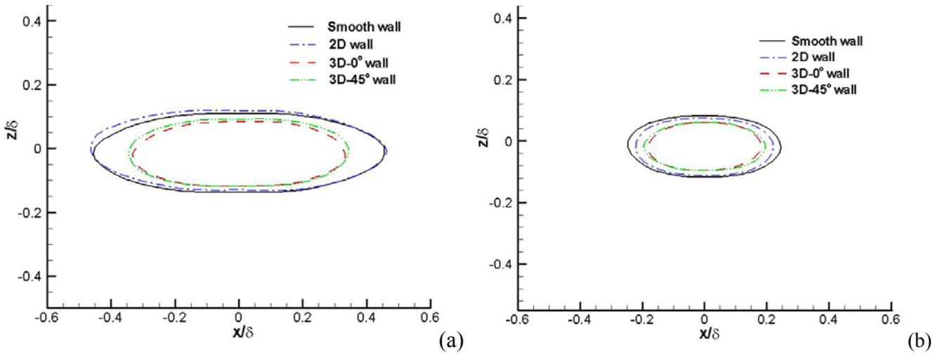
Fig.11 Two point streamwise velocity auto-correlation function  $\rho_{u'u'} = 0.6$  in the planes  $y/\delta = 0.2$  (a) and  $y/\delta = 0.3$  (b).
