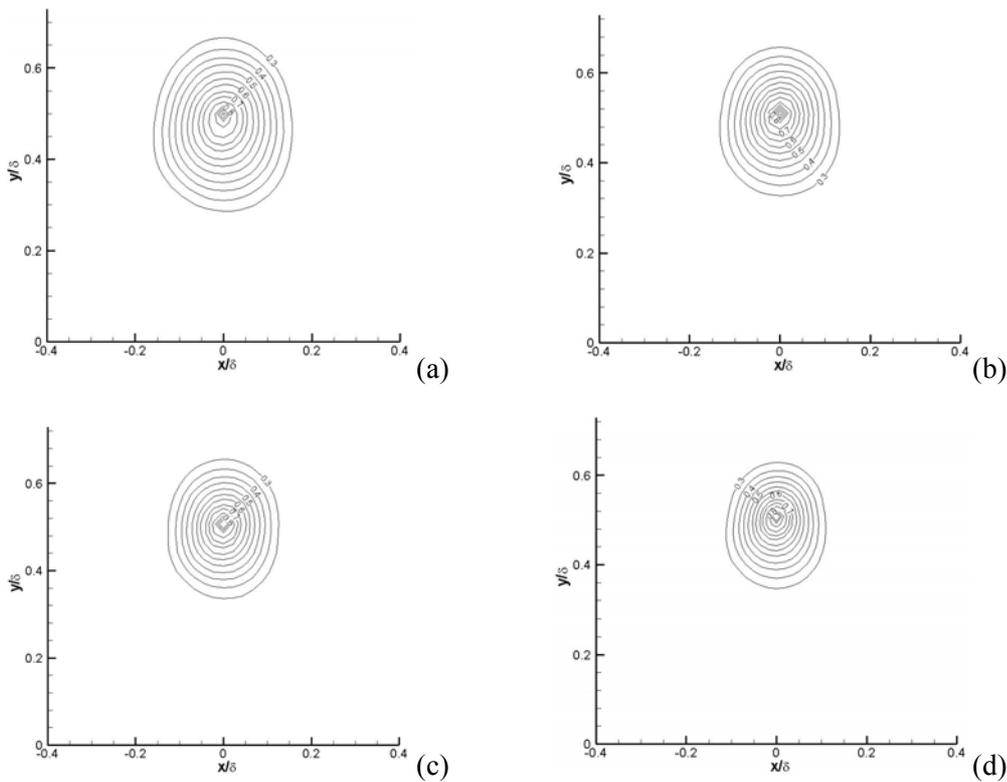
Fig. 8 Contours of constant values of the two point wall normal velocity auto-correlation function.  $(y/\delta)_{ref.} = 0.5$ . (a): smooth wall; (b): 2D wall; (c): 3D-0° wall; (d): 3D-45° wall
