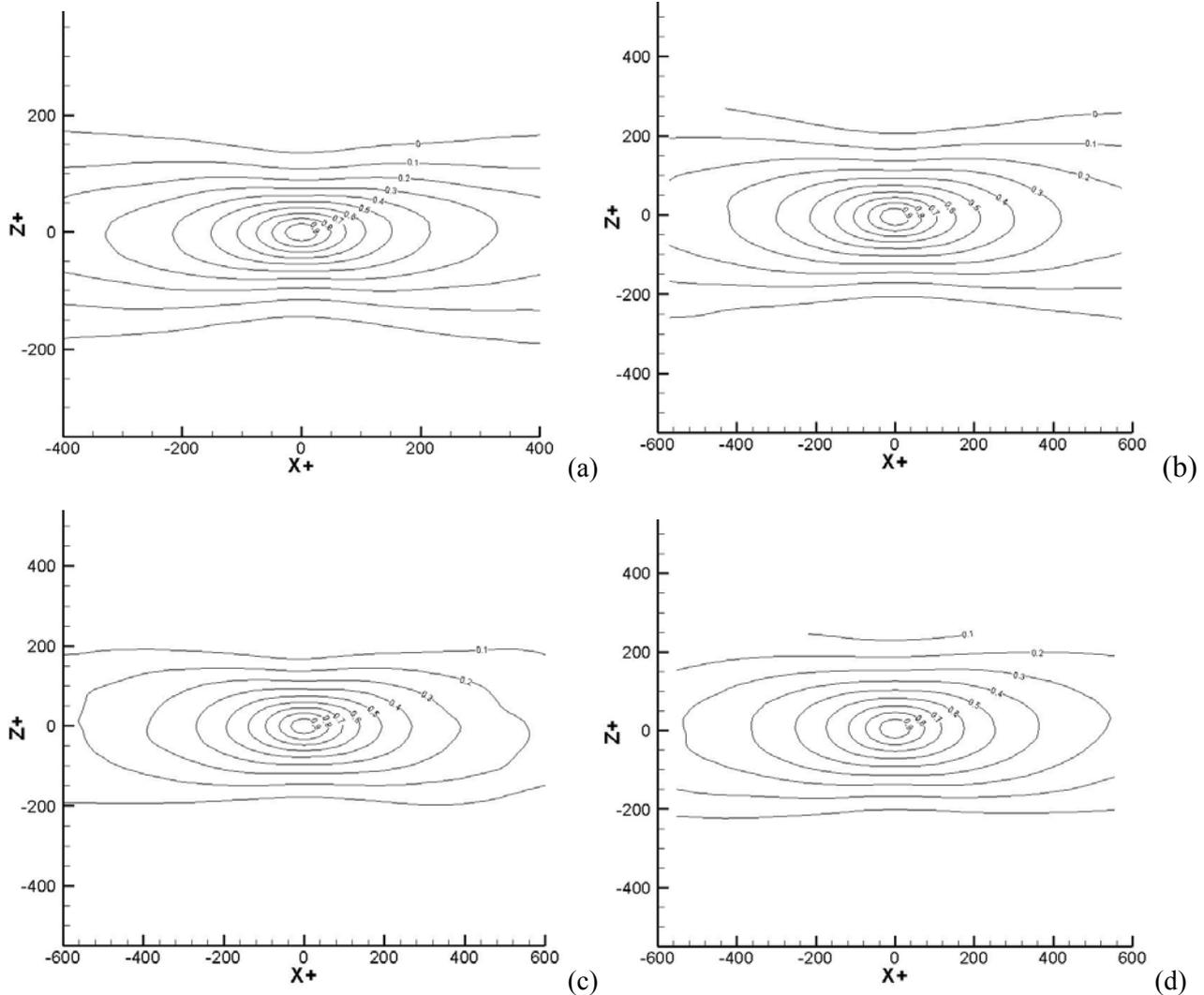
Fig.10 Two point streamwise velocity auto-correlation function in the plane  $y/\delta = 0.3$ . (a): smooth wall, (b): 2D wall, (c): 3D-0° wall, (d): 3D-45° wall.
