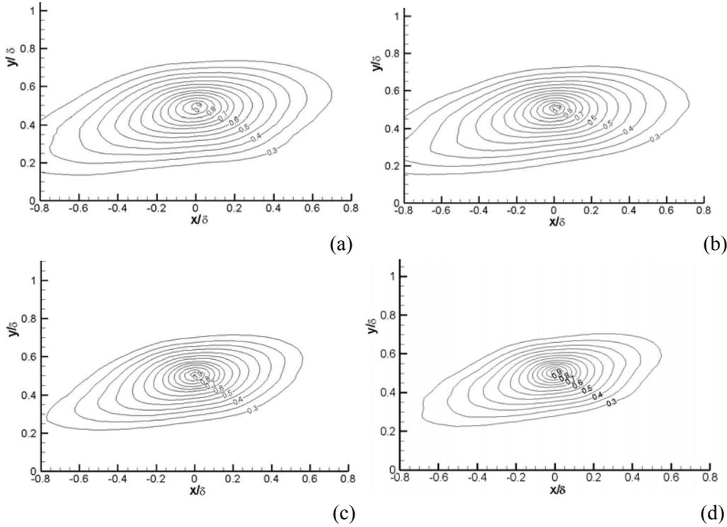
Fig. 7 Contours of constant values of the two point streamwise velocity auto-correlation function.  $(y/\delta)_{ref.} = 0.5$ . (a): smooth wall; (b): 2D wall; (c): 3D-0° wall; (d): 3D-45° wall.
