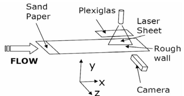
Fig.1 Experimental set-up for measurements in the plane (x,y).
