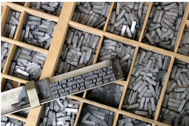
Fig. 2. Letter punches (movable types)
