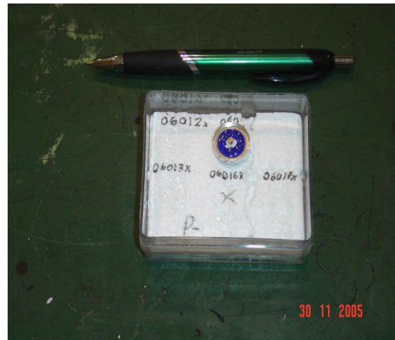
Fig.1 The CATGAS Conductometric Gas Sensor
