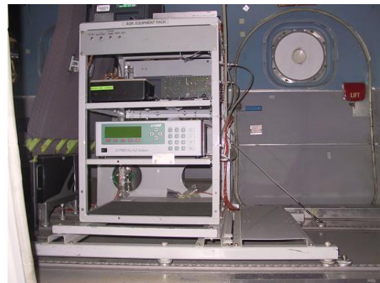
Fig. 7 The On-board LiCor LI-7000 CO 2 Analyser
