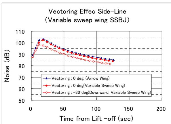
Fig. 17 Sideline noise reduction by Variable sweep wing
