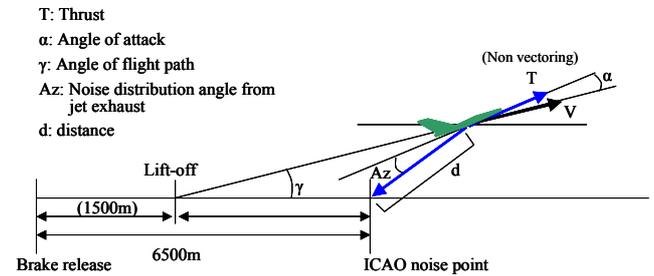
Fig. 4 Take-off flight path and noise point
