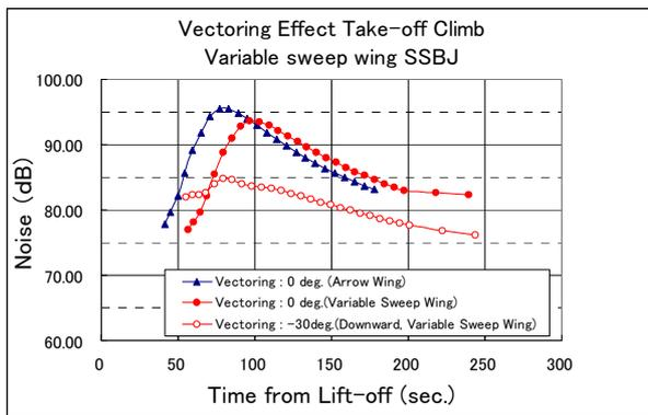
Fig. 16 Take off noise reduction by Variable sweep wing
