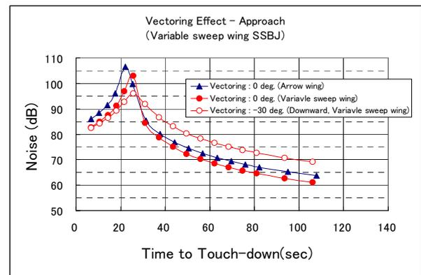
Fig. 18 Approach noise reduction by Variable sweep wing
