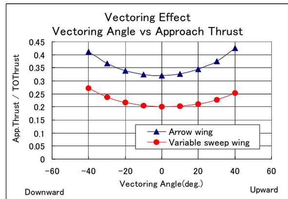
Fig. 8 Thrust level to keep 3deg glide slope
