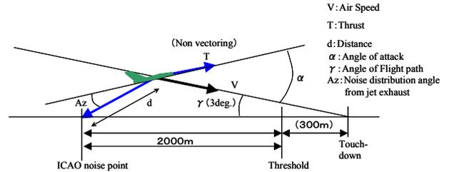
Fig. 7 Approach flight path and noise point
