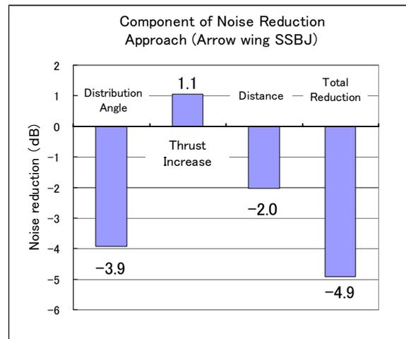
Fig. 15 Component of approach noise reduction
