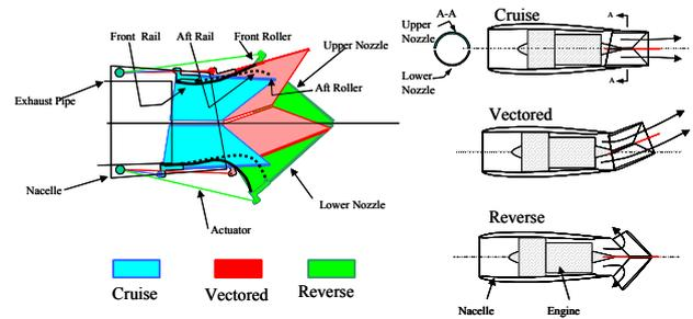
Fig. 20 Vectoring nozzle concept
