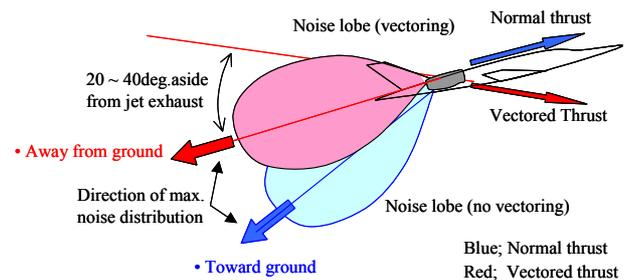
Fig. 1 Concept of the thrust vectoring
