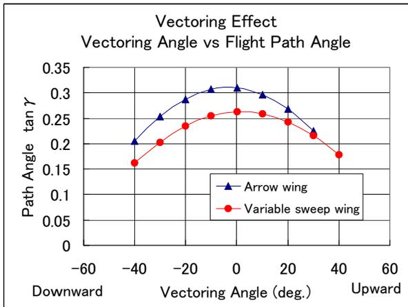
Fig. 6 Climb path and vectoring angle
