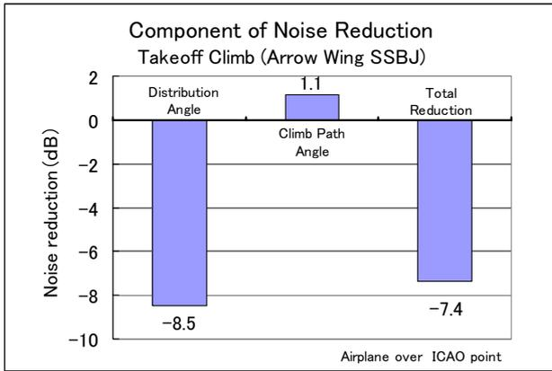
Fig. 12 Component of take off noise reduction
