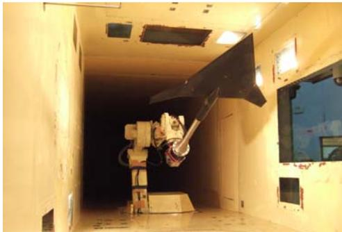
Fig.2 2m x 2m circuit type low-speed wind tunnel
