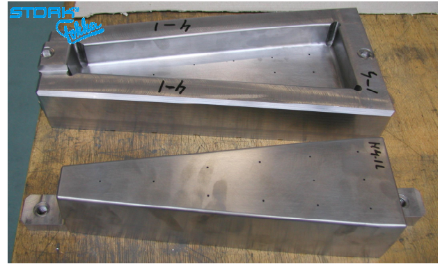
Figure 2 The mould set used to press a rib
