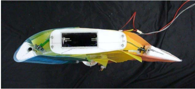
Fig. 9. Model cross section with leading edge and trailing edge deflection
