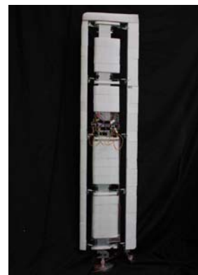
Fig. 7. Wind tunnel test model inside view
