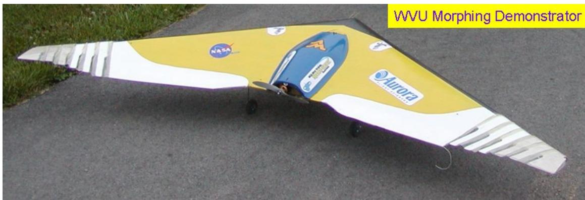
Fig. 10. WVU 7' morphing flight demonstrator ready for flight.
