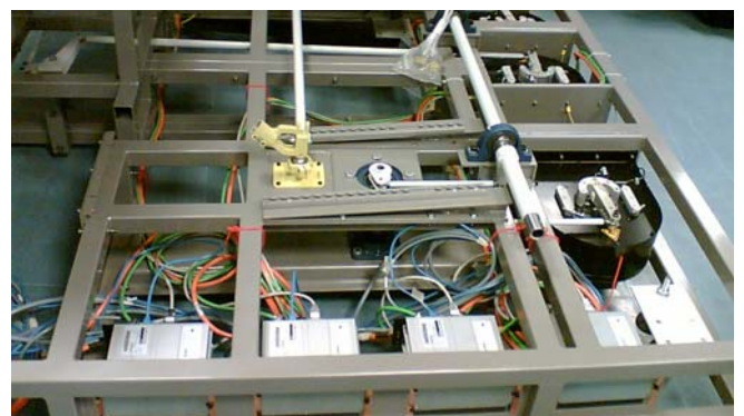
Fig. 7 – Force feedback motors and controllers
