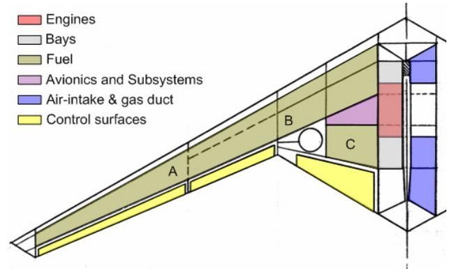
Fig. 6. Internal subsystems arrangement
