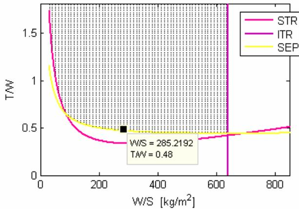
Fig. 4. Constraints diagram; AR 15, BPR 6
