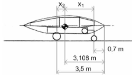
**Fig. 8. Landing gear: longitudinal location check**
