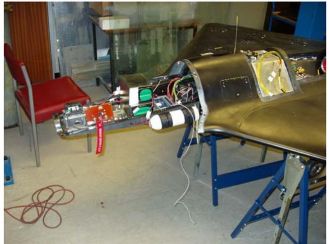
'Fig. 2. The Eclipse UAV new FCS and battery packs'
