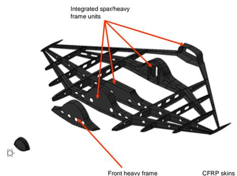
‘Fig. 10. Main Structural Components’
