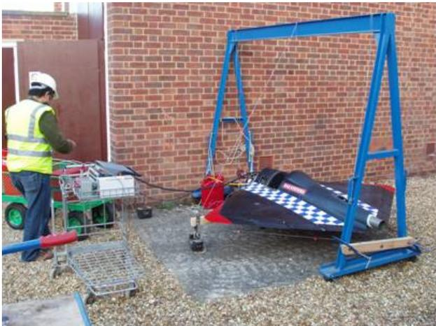
‘Fig. 4. The Eclipse UAV propulsion system test’
