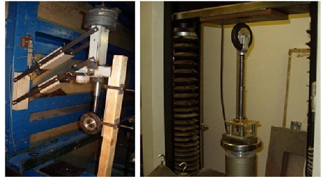
‘Fig. 5. The Eclipse UAV Main and nose Undercharge tests’
