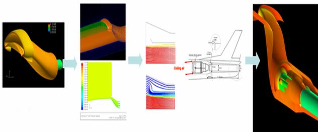
‘Fig. 3: The Eclipse UAV propulsion system evaluation process’
