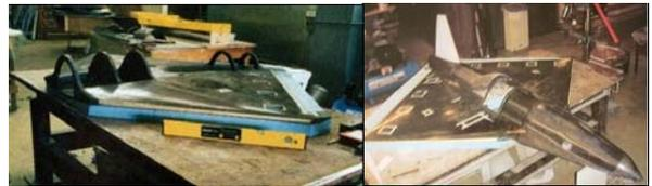
‘Fig. 1. The original Eclipse UAV during manufacturing’
