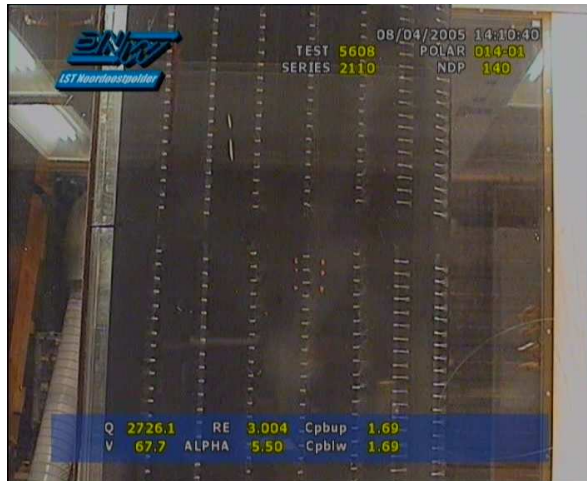
Fig. 7. Tuft pattern at \alpha=5.5^\circ
