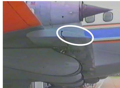
Fig. 2. DLC-flaps mounted on the ATTAS landing flap
