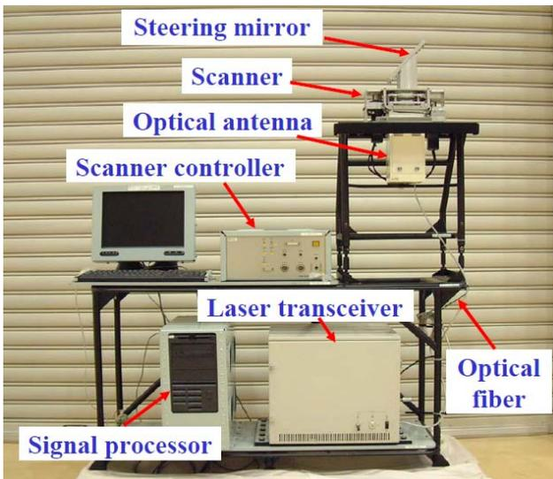
Fig. 4. 1NM Class LIDAR
