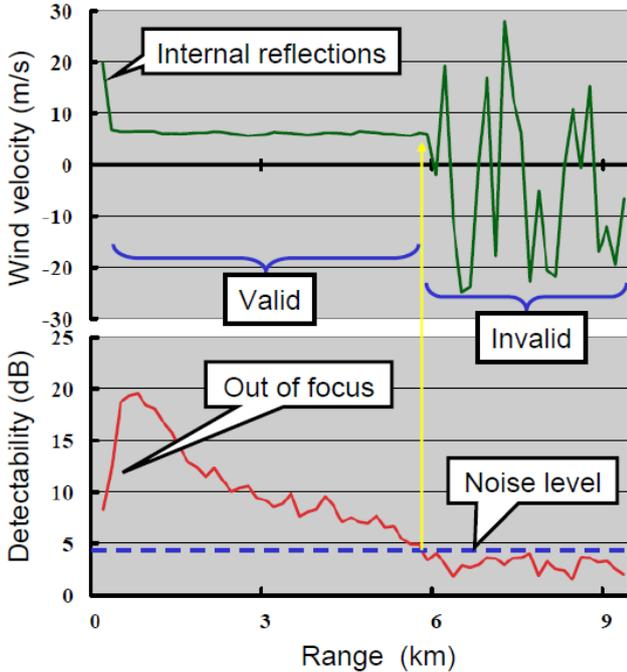
Fig. 7. In-Flight Measured Data by the 3NM Class LIDAR
