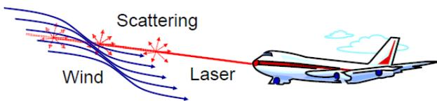
Fig. 2. Concept of an Onboard Doppler LIDAR
