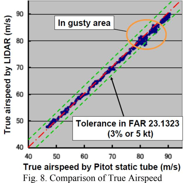
Fig. 8. Comparison of True Airspeed
