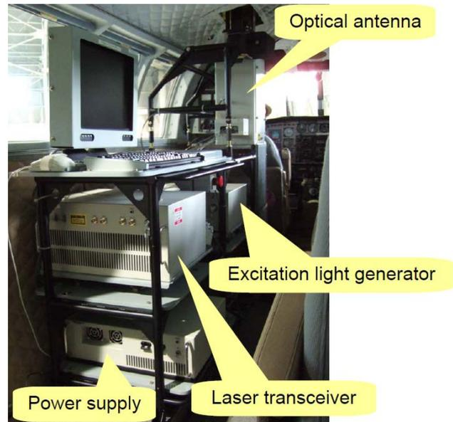
Fig. 6. Installation of the Experimental System
