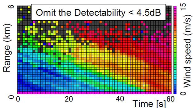
Fig. 10. Wind Measurement Cleaned Data
