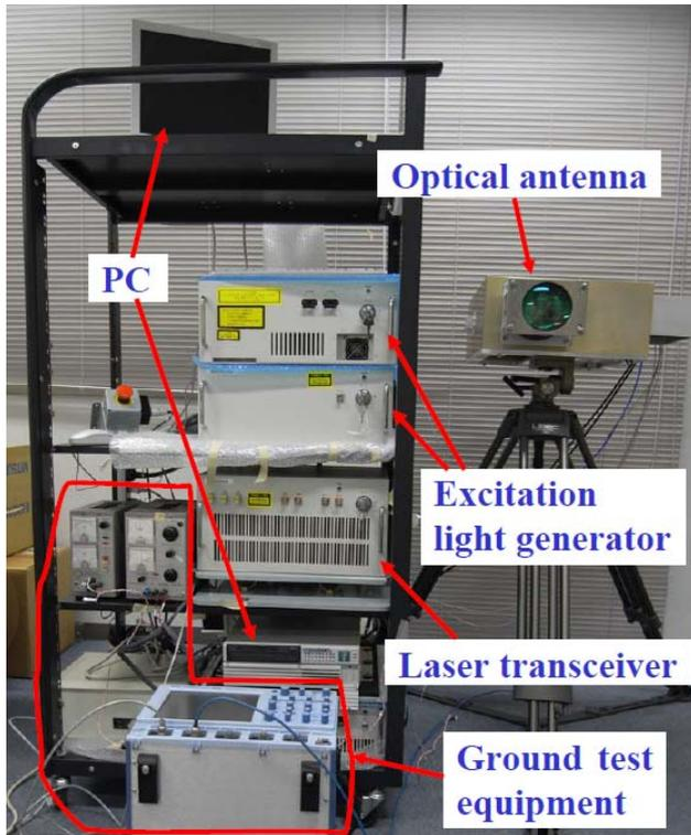
Fig. 12. 5NM Class LIDAR
