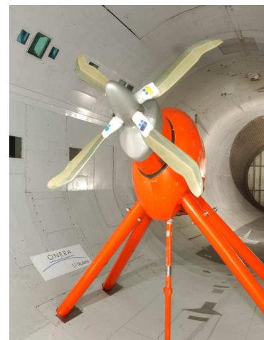
Fig. 11: The Adyn rotor on the Eurofar hub in the S1MA wind-tunnel
