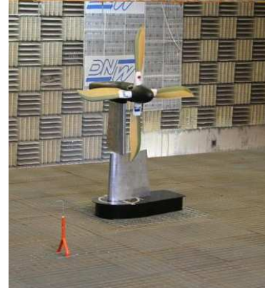
Fig. 10: The Tilttaero rotor on the Tilttaero model in the DNW-LLF wind-tunnel
