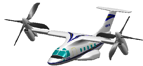
Fig. 1: The ERICA half tilt-wing tilt-rotor of Agusta
