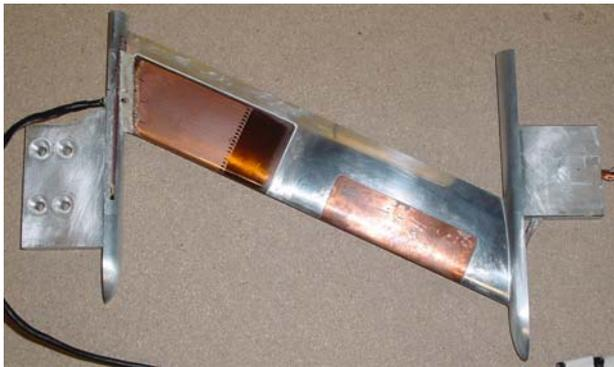
Fig. 12 Swept airfoil model equipped with surface hot film array (DLR, left) and surface hot wire array (TU Berlin, right)
