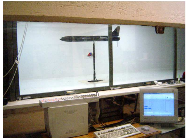
Fig. 6 Wind tunnel setup with the research base aircraft model [6].
