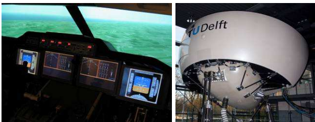
Fig. 9. SIMONA cockpit configuration for the GARTEUR FM-AG(16) piloted simulator campaign.
