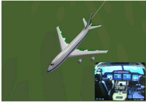
Fig. 15. FM-AG(16) piloted simulation showing aircraft with separated right-wing engines (Flight 1862 scenario).
