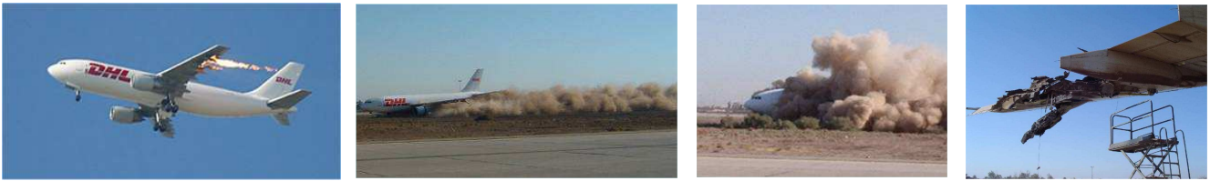
Fig. 1. Emergency landing sequence using engines only and left wing structural damage due to surface-to-air missile impact, DHL A300B4-203F, Baghdad, 2003.
