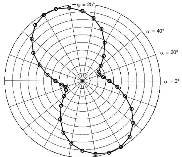
Figure 10: Twist of a winglet correlated to the orientation of a SMA actuated orthotropic composite material
