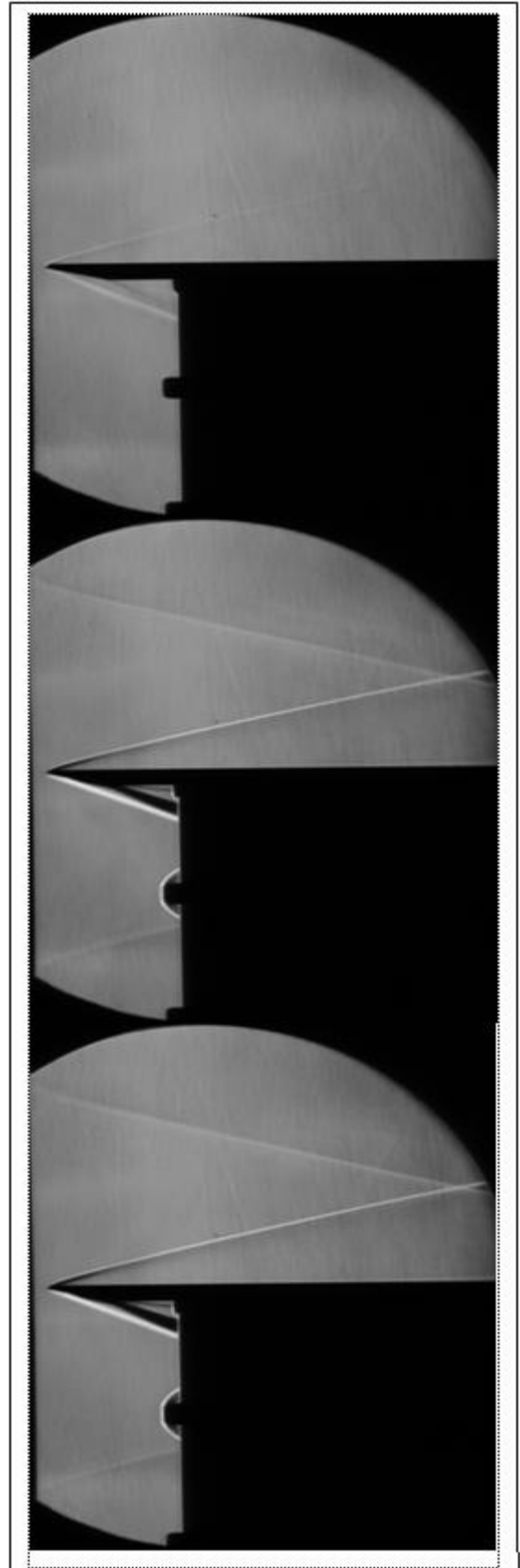
Figure 5 Schlieren visualization of flowfield during test run
