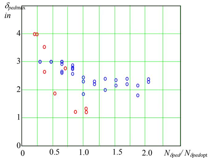
Fig. 6. Maximum pedal deflections for different values of directional control sensitivity.
