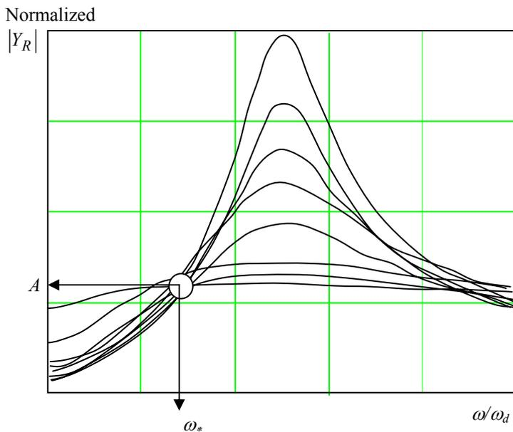
Fig. 3. Amplitudes of  $Y_R$  transfer function for different dynamic configurations at the optimum yaw control sensitivity.
