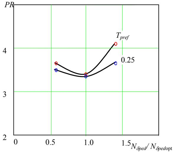
Fig. 10. Effect of a prefilter time constant on the optimum directional control sensitivity.
