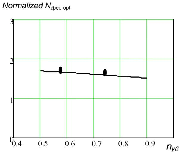
Fig. 8. Optimum control sensitivity as a function of parameter  $n_{y\beta}$
