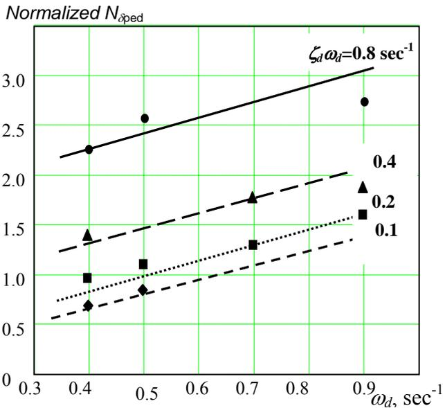
Fig. 7. Optimum control sensitivity as a function of dynamic characteristics.
