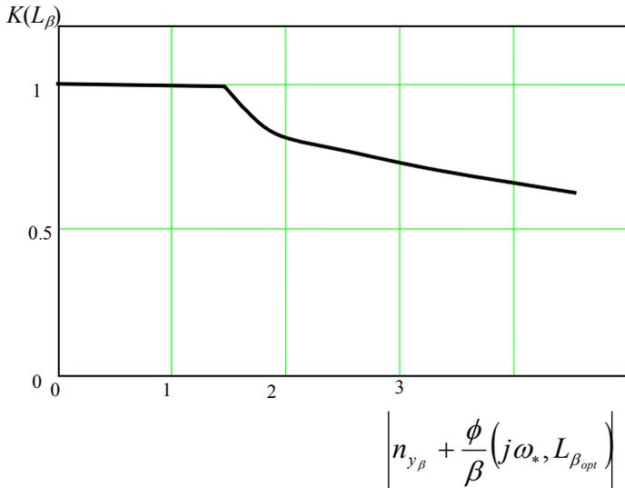
Fig. 2. Diagram to determine the effect of  $L_\beta$  on the optimum directional control sensitivity.
