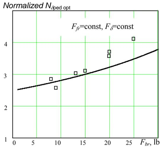
Fig.13. Effect of breakout on the optimum yaw control sensitivity.
