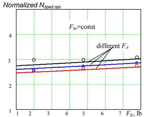
Fig. 12. Effect of friction on the optimum yaw control
