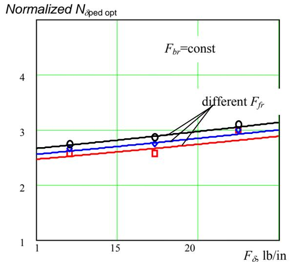
Fig. 11. Effect of spring gradient on the optimum yaw control sensitivity.
