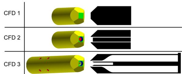
**Fig 4. The Pitot Probe Shape for CFD Analysis**
