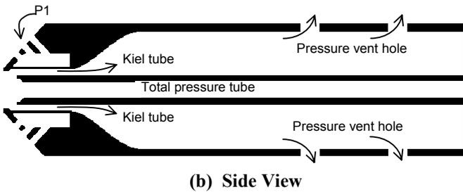
**Fig 2. The Pitot Probe with Five-Hole Pyramidal Head**
