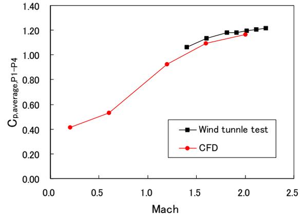
Fig 13. Mach Number Effect of Wind Tunnel Test and CFD at  $\alpha=0$  degree
