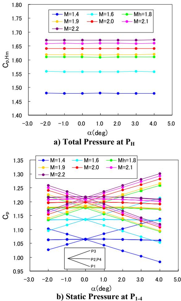
Fig 12. Mach Number Effect of Wind Tunnel Test
