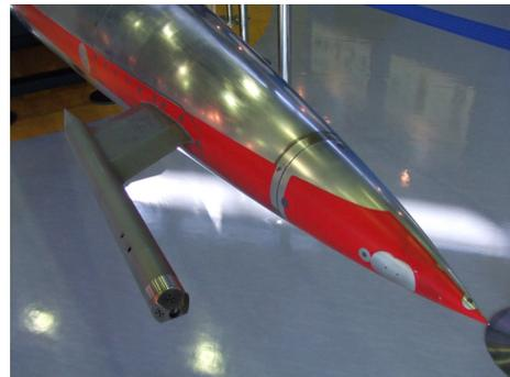
Fig 1. The Pitot Probe of NEXST-1
