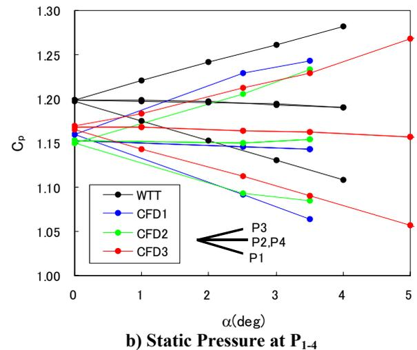
Fig 6. Comparison the Wind Tunnel Test and CFD
