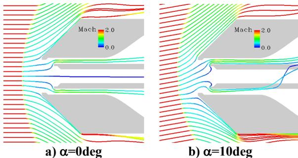
**Fig 15. Mach Number and Stream line Around Pressure hole of CFD ( $\alpha=0\text{deg}$ ,  $\alpha=10\text{deg}$ )**
