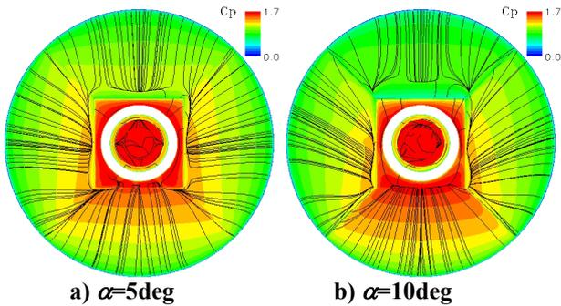
**Fig 14.  $C_p$  Distribution and Surface flow of CFD ( $\alpha=5\text{deg}$ ,  $\alpha=10\text{deg}$ )**
