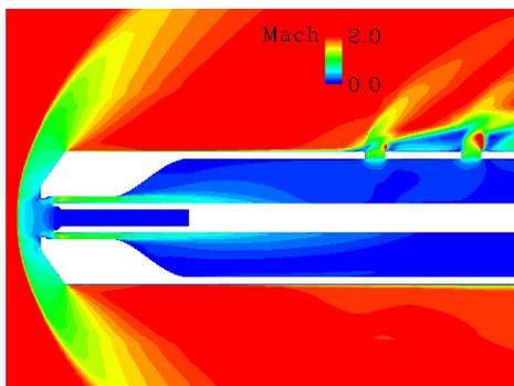
Fig 10. Mach Distribution of CFD3 at  $\alpha=0deg$  on the cross section including the center and pressure vent hole
