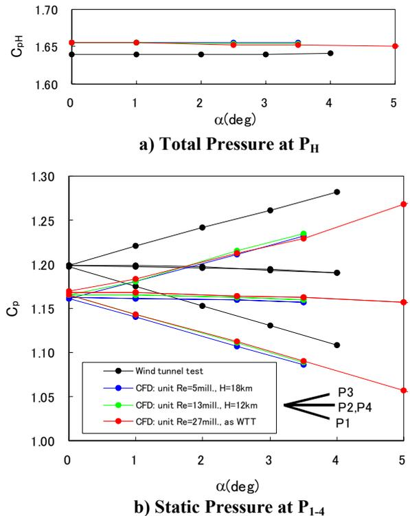
Fig 11. Comparison of the Wind Tunnel Test and CFD on the different Reynolds number.
