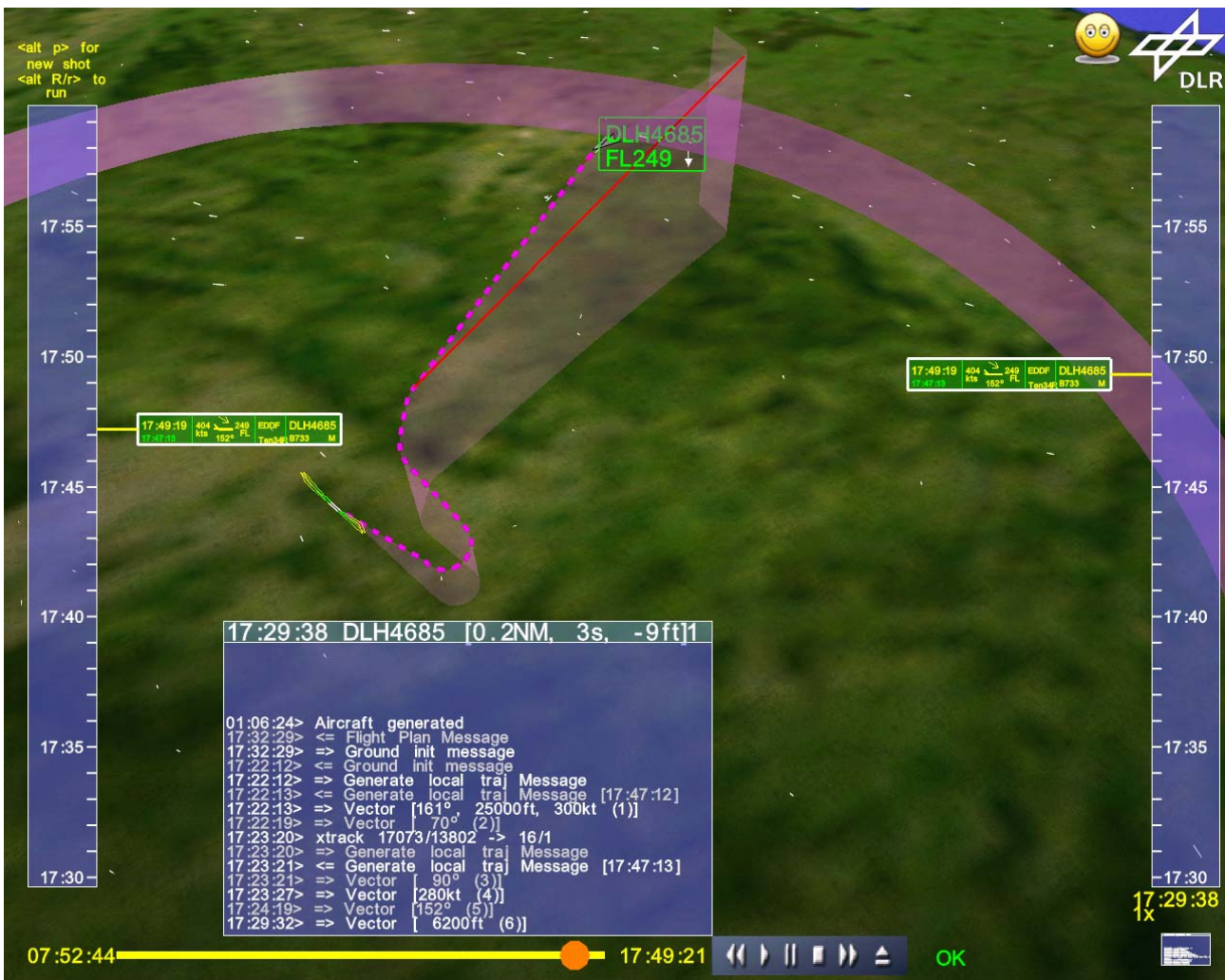
Fig. 9: Ground based 4D guidance for one aircraft
