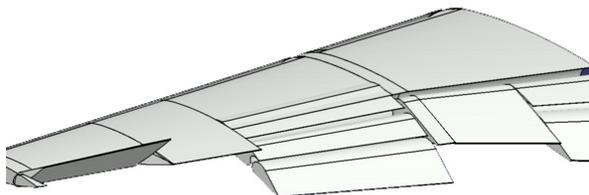
Figure 5 –Wing with high lift devices deployed
