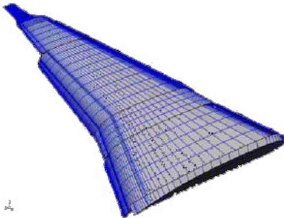
Figure 10 – Wing in takeoff configuration - superficial mesh
