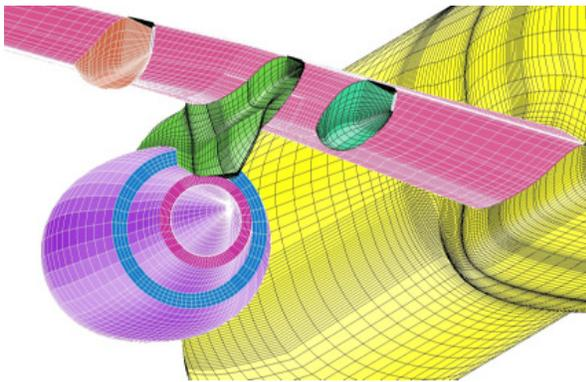
Figure 9 – Under-wing configuration with FTF
