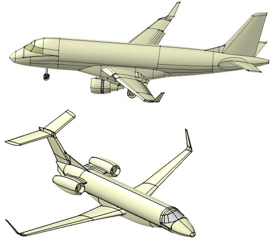
Figure 7 – Full aircraft geometries created with GMA
