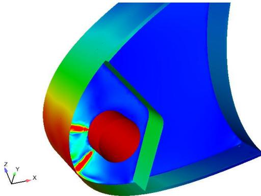
Figure 14 – D-bay temperature field obtained after the application of the GMA plus FLUENT set up analysis tool.
