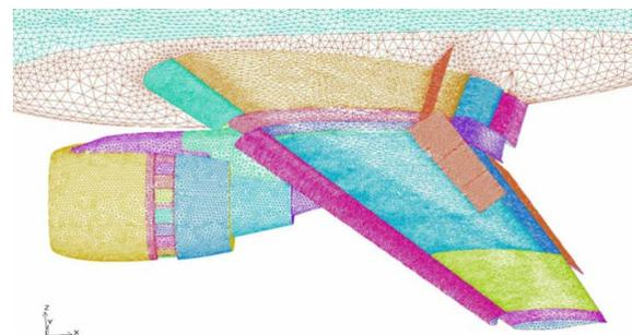
Figure 8 – Landing configuration with spoiler deflected
