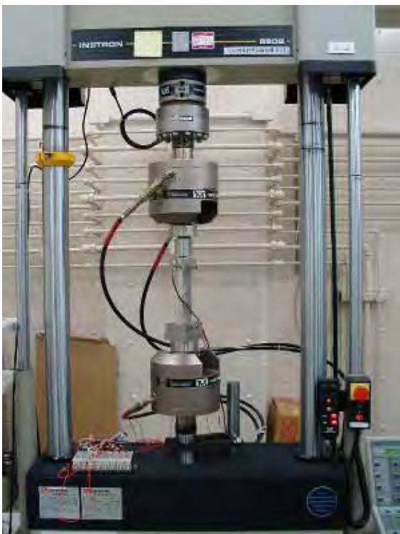
Fig. 8. Test Set-up of the Quasi-Static Test
