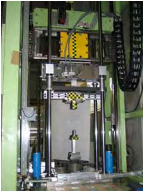
Fig. 7. Loading Frame of the Impact Tests with Light Weight Holder
