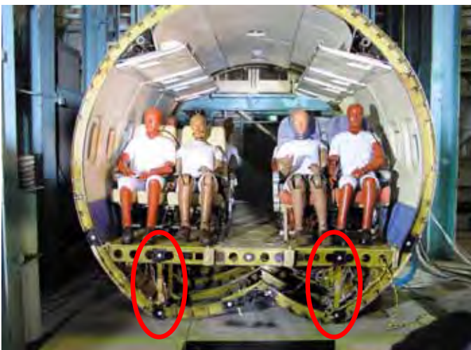
Fig. 1. Post Test Photo of YS-11 Fuselage Section Vertical Drop Test.
