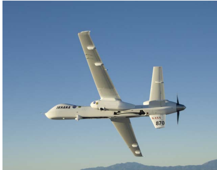
Fig. 6. The Ikhana aircraft carrying the fire pod.
