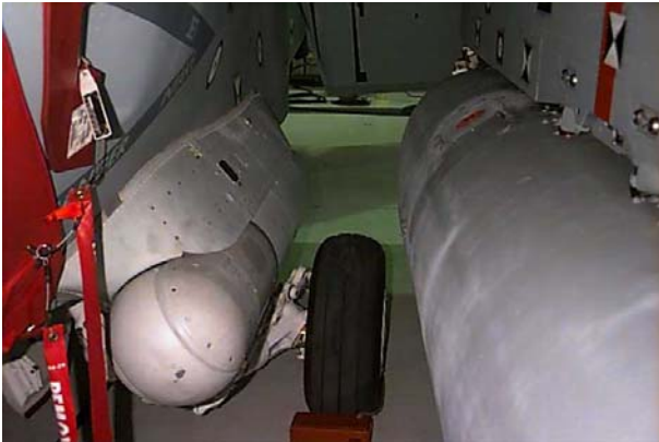
Fig 1. TFLIR pod mounted on F-18C
