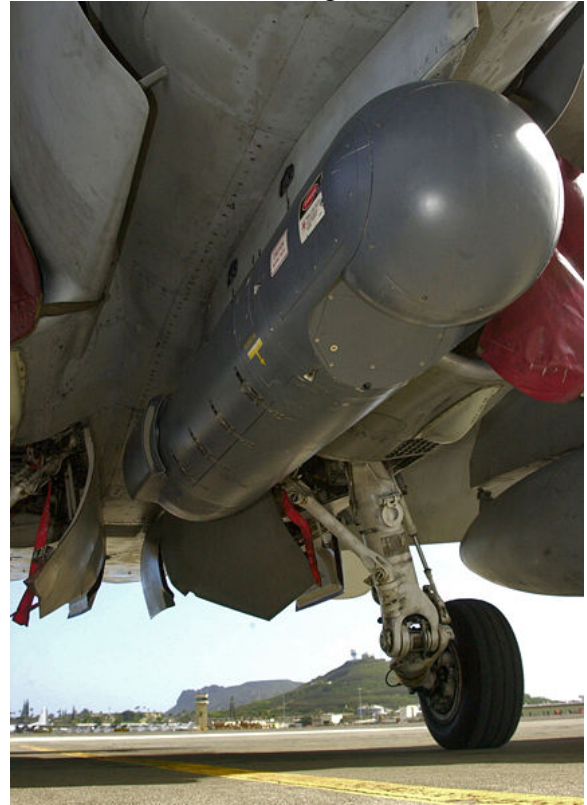
Fig 16. Litening pod on underbelly of F/A-18A Hornet
