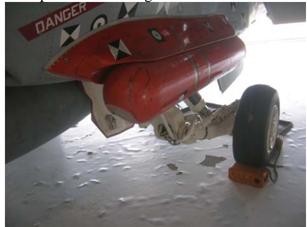
Fig 2. ATFLIR pod mounted on F-18C [2]
