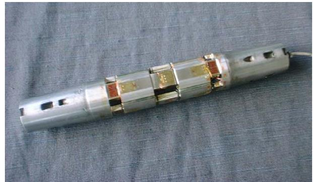
Fig. 4. Force balance with semiconductor strain gauges
