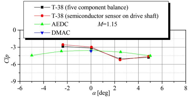
Fig. 14. Roll – damping derivative for the MBFM model at the  $M = 1.15$
