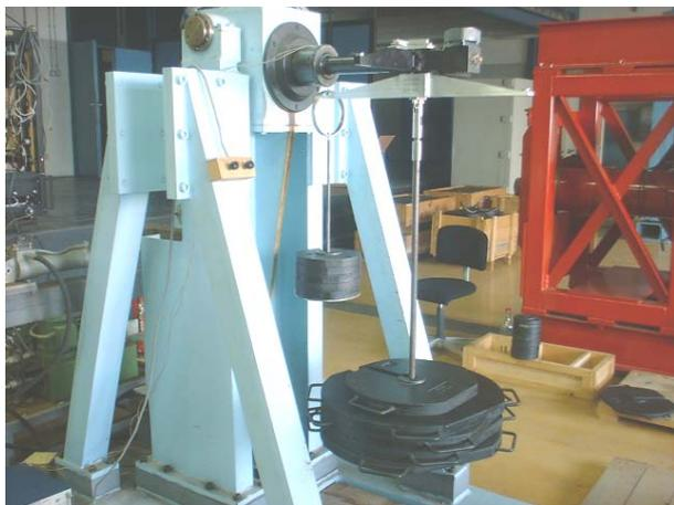
Fig. 6. Strain gauge-balance on the VTI six-component calibration ring
