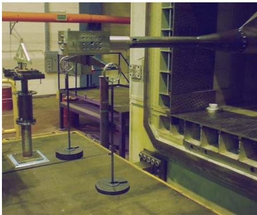
**Fig. 8.** Calibration of the excitation moment sensor
