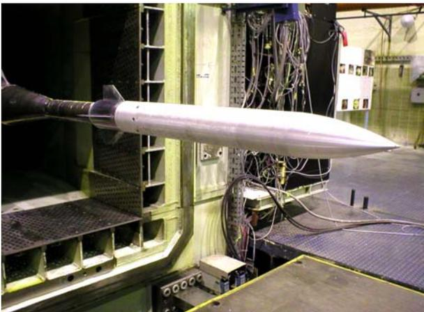
Fig. 12. MBFM model in the T-38 test section
