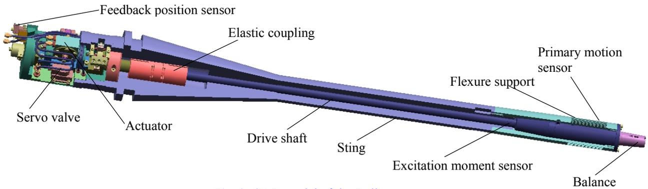
Fig. 2. CAD model of the Roll apparatus
