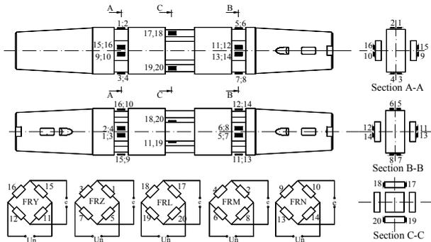
Fig. 5. Position of the measuring section and the measuring bridges
