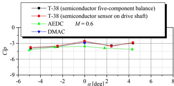
Fig. 13. Roll – damping derivative for the MBFM model at the  $M = 0.6$
