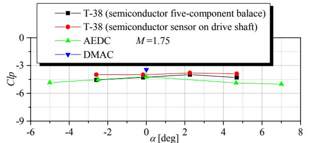
Fig. 15. Roll – damping derivative for the MBFM model at the  $M = 1.75$
