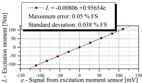
**Fig. 9.** Result of the excitation moment sensor calibration
