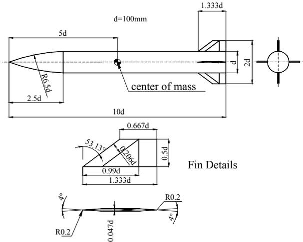
Fig. 11. Basic dimension of the MBFM model
