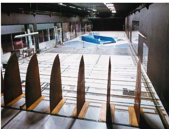
Fig. 8. Turbulent Boundary Layer Generator and the Model in the Wind Tunnel
