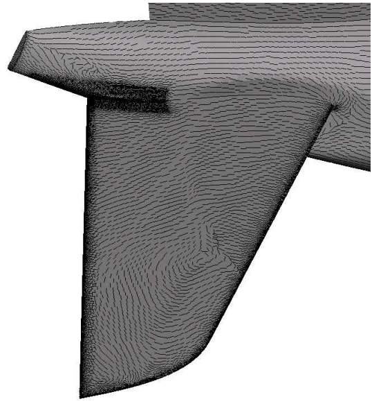
Fig. 12 Surface flow pattern for unsealed gap. Steady computation, Re = 38 \cdot 10^6 , \alpha = \alpha_2 .
