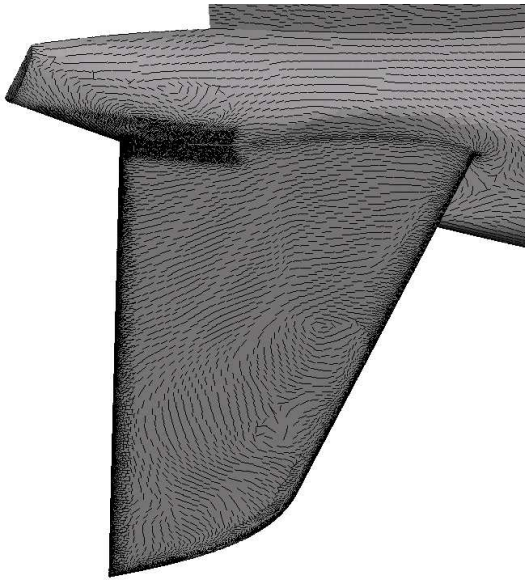
Fig. 10 Surface flow pattern for sealed gap. Steady computation, Re = 38 \cdot 10^6 , \alpha = \alpha_2 . In the gap region the velocity vectors are not visible due to high node density.
