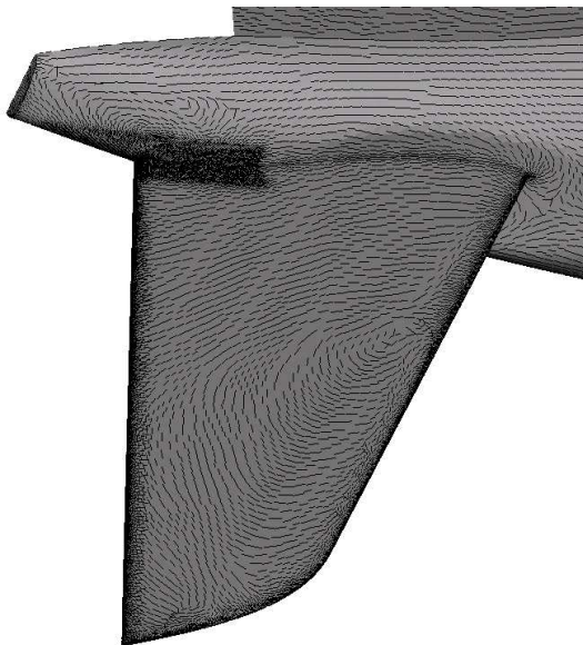
Fig. 11 Surface flow pattern for sealed gap. Unsteady computation, Re = 38 \cdot 10^6 , \alpha = \alpha_2 .
