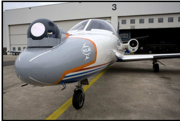
Fig. 7. Toplite II installation in NLR Citation
