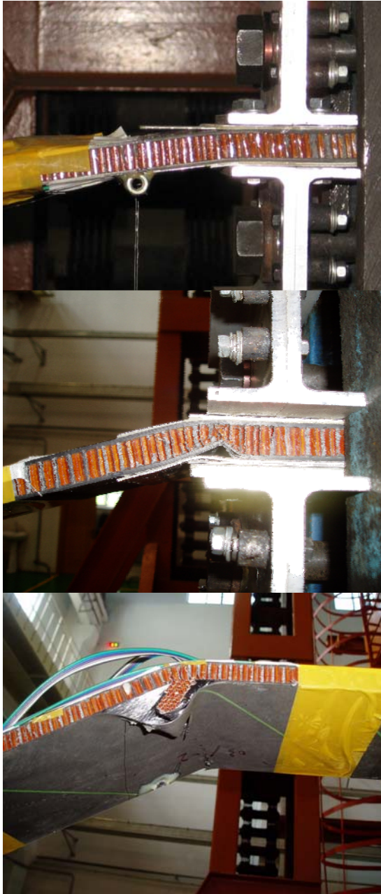
Fig 9 The failure modes of experiment samples
