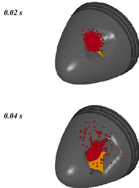
**Fig. 6. Birdstrike onto a composite spinner.**
