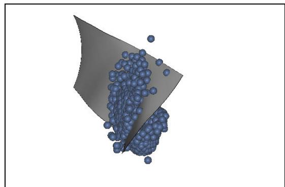
Fig. 2. Birdstrike onto a blade.
