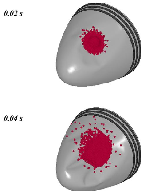
**Fig. 7. Birdstrike onto a metallic spinner.**
