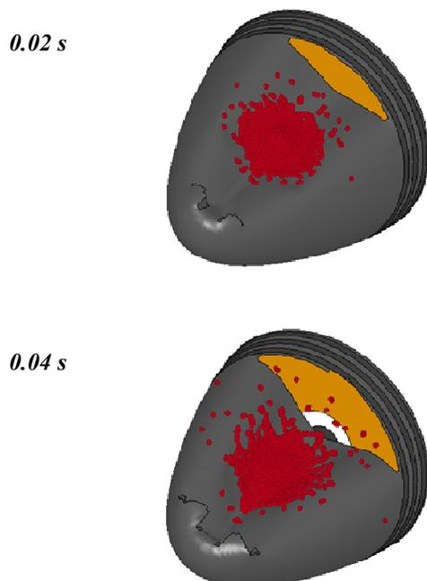
**Fig. 5. Birdstrike onto a motionless spinner.**
