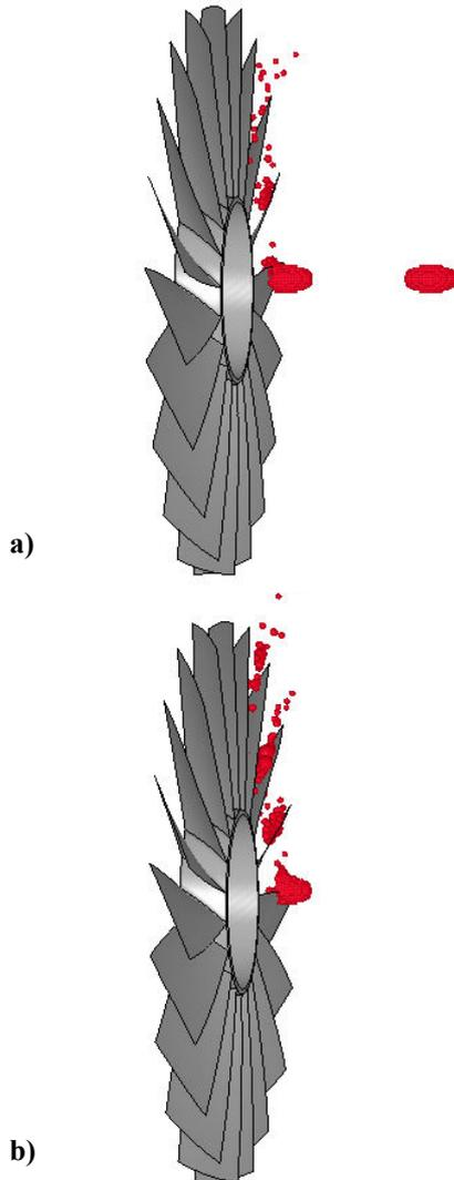
**Fig. 3. Bird impact onto a low-pressure fan blade.**
