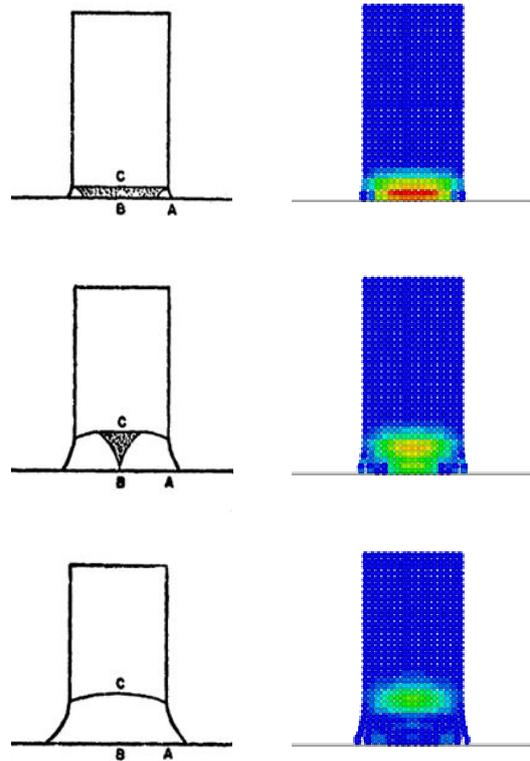
Fig. 1. Shock and release in a bird impact [2].
