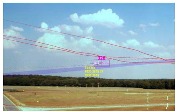
Fig. 4: Screenshot of camera no. 4 (= E) display showing augmentation during landing. Superimposed glide path (blue), GPS-trajectories (red), multilateration position (yellow, from transponder) and automatic movement detection (violett square).
