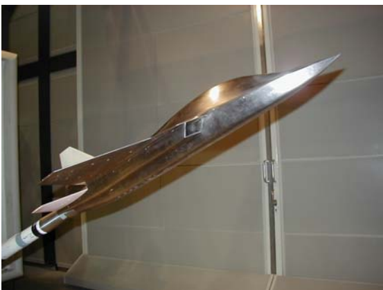
c) Model mounted in the test section; \alpha = 25^\circ .
