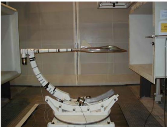
b) Model mounted in the test section; \alpha = 0^\circ .
