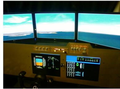
Fig. 7 PC-based Simulator.
