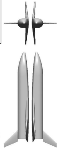
Fig. 2. LGBB bimese wing-body configuration in belly-to-belly arrangement.
