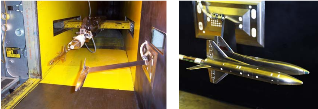
Fig. 6. Photographs of the LBG configuration installed in Test Section 2 of the NASA LaRC UPWT.
