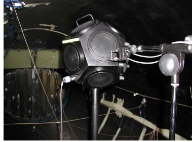
Fig. 3. Volume velocity source (B&K4296 "OmniPower")
