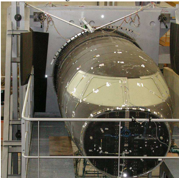
Fig. 1. FUBACOMP barrel with acoustic array
