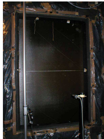
Fig. 8. Dassault set-up for TL measurement of the FUBACOMP panel
