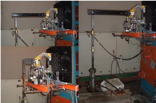
Fig. 26. Combination of bending and shear of No.6 part
