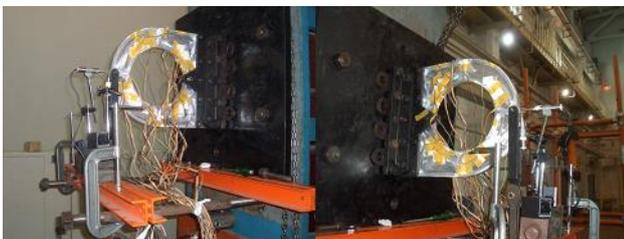
Fig. 18. Shear load process of No. 3 test part
