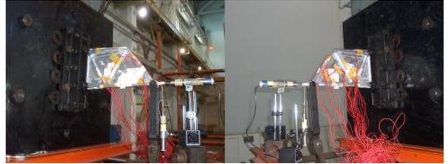
Fig. 30. Shear load process of No. 8 test part
